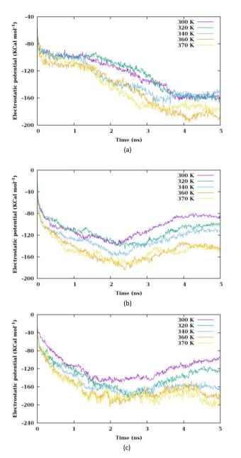
Fig. 7 Electrostatic interaction potential between the nanosheet and membrane *versus* the simulation time at different values of temperature for (a) CF1, (b) CF2 and (c) CF3 configurations.
