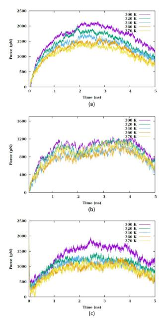
Fig. 2 Pulling forces versus the simulation time at different values of temperature (i.e., 300, 320, 340, 360 and 370 K) for (a) CF1, (b) CF2 and (c) CF3 configurations.
