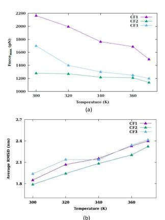
**Fig. 3** (a) Maximum pulling force at different values of temperature for CF1, CF2 and CF3 configurations. (b) Average Root Mean Square Deviation of CF1, CF2 and CF3 configurations at different values of temperature.
