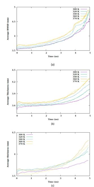
**Fig. 8** Average thickness of membrane *versus* the simulation time at different values of temperature for (a) CF1, (b) CF2 and (c) CF3 configurations.
