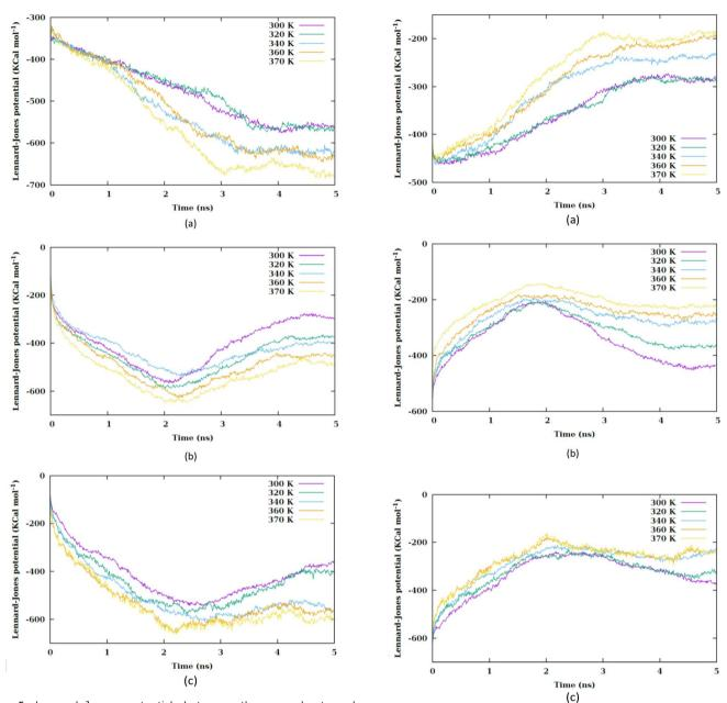
Fig. 5 Lennard-Jones potential between the nanosheet and membrane *versus* the simulation time at different values of temperature for (a) CF1, (b) CF2 and (c) CF3 configurations.
