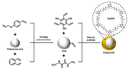
Fig. 1 Schematic preparation of PAD@COF.
