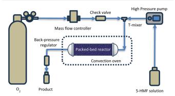
Fig. 1 The continuous process for DFF production.
