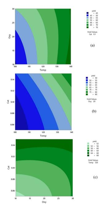
Fig. 8 Response surface and contour plots illustrating the yield of DFF utilizing the Box–Behnken design, achieved by plotting (a) oxygen flow rate *versus* reaction temperature, (b) catalyst amount *versus* reaction temperature, and (c) catalyst amount *versus* oxygen flow rate.
