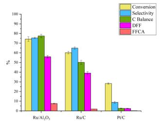
Fig. 5 Impact of catalyst types on reaction performance. Experimental conditions: temperature maintained at 120 °C, 5-HMF solution concentration of 5 g  $L^{-1}$ , flow rate of 0.06 ml min $^{-1}$  for 5-HMF solution, acetonitrile utilized as the solvent, oxygen gas flow rate set at 10 ml min $^{-1}$ , and catalyst quantity of 0.05 g.
