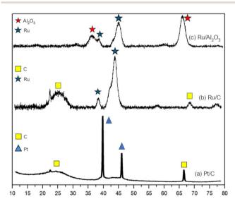
Fig. 2 The XRD pattern of catalyst (a) Pt/C, (b) Ru/C and (c) Ru/Al<sub>2</sub>O<sub>3</sub>.
