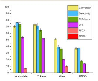
Fig. 6 Impact of solvent on reaction performance. Experimental conditions: temperature maintained at 120 °C, 5-HMF solution concentration of 5 g L $^{-1}$ , flow rate of 0.06 ml min $^{-1}$  for 5-HMF solution, oxygen gas flow rate set at 10 ml min $^{-1}$ , and catalyst quantity of 0.05 g (Ru/Al $_2$ O $_3$ ).
