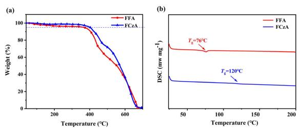
Fig. 2 (a) TGA and (b) DSC curves of FFA and FCzA.
