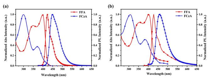
Fig. 4 (a) UV-vis spectra and PL spectra in THF ( $10^{-5}$  M), and (b) UV-vis spectra and PL spectra of FFA and FCzA in the film state.
