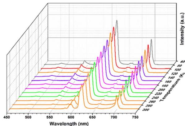
Fig. 4 Temperature-dependent emission spectra of Eu@SNNU-325 recorded in the range of 80–300 K.
