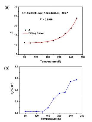
Fig. 5 (a) Temperature-dependent emission intensity ratio  $\Delta$  ( $I_{618}/I_{544}$ ) and the fitted curve of Eu@SNNU-325 from 80 to 260 K. (b) Temperature-dependent relative sensitivity ( $S_r$ ) of Eu@SNNU-325.
