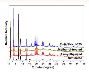
**Fig. 1** PXRD patterns of the simulated, as-synthesized SNNU-325, methanol-treated SNNU-325 and Eu@SNNU-325.
