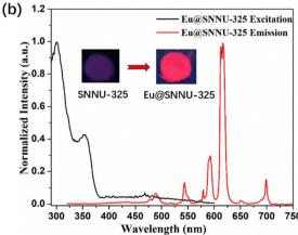
Fig. 3 Excitation and emission spectra of SNNU-325 ( $\lambda_{ex}=353$  nm) (a) and Eu@SNNU-325 ( $\lambda_{ex}=300$  nm) (b) (insets show the photographs under 254 nm UV light).
