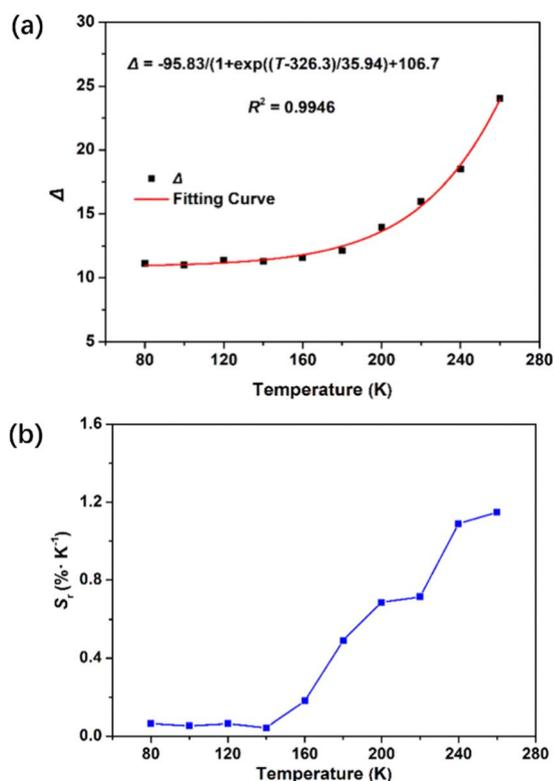
Fig. 5 (a) Temperature-dependent emission intensity ratio  $\Delta$  ( $I_{618}/I_{544}$ ) and the fitted curve of Eu@SNNU-325 from 80 to 260 K. (b) Temperature-dependent relative sensitivity ( $S_r$ ) of Eu@SNNU-325.
