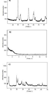
Fig. 3 XRD patterns (a) SZ, (b) Al-MCM-41 and (c) montmorillonite modified before being reused.
