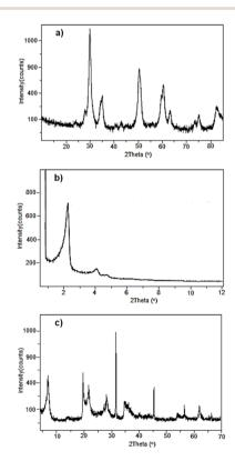
Fig. 1  $\,$  XRD patterns of (a) SZ, (b) Al-MCM-41 and (c) montmorillonite modified with CF $_3 SO_3 H.$
