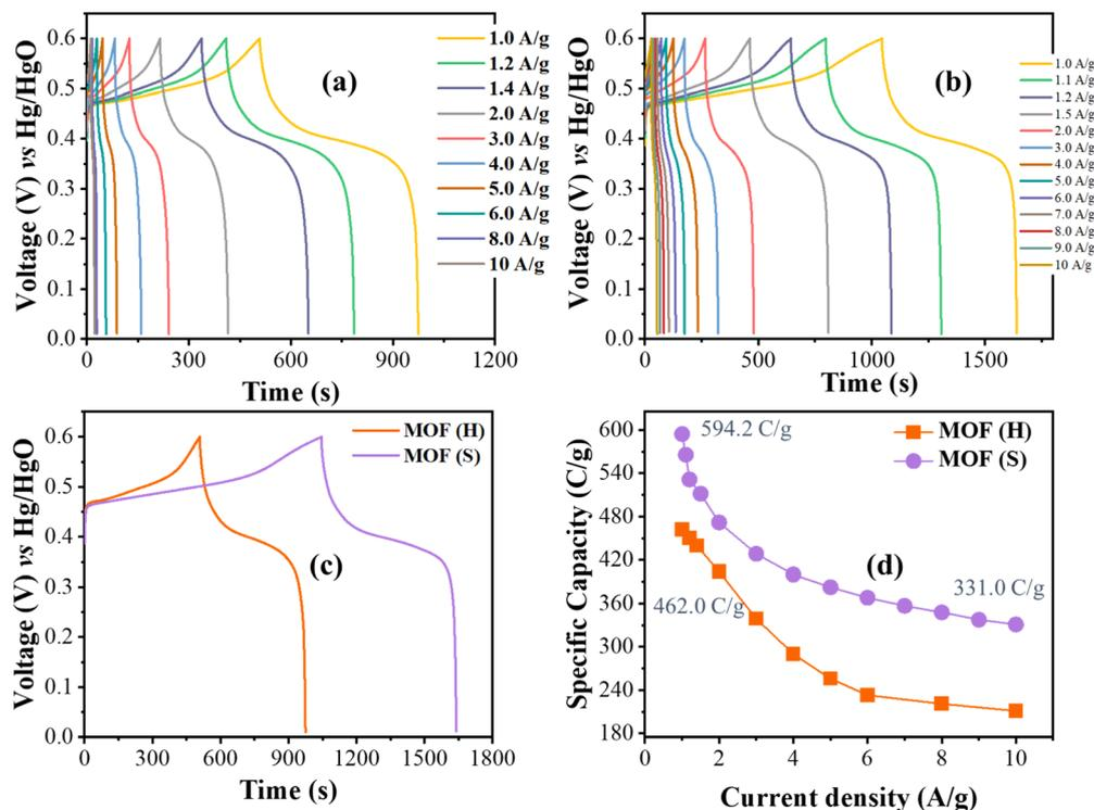
Fig. 5 (a and b) GCD results recorded at different current densities (1–10 A g<sup>-1</sup>) for Q1 and Q2 electrodes, respectively, (c) Comparison of GCD at 1 A g<sup>-1</sup> for comparative analysis, (d)  $Q_s$  calculated from the GCD results, showing the dominant performance of Q2.
