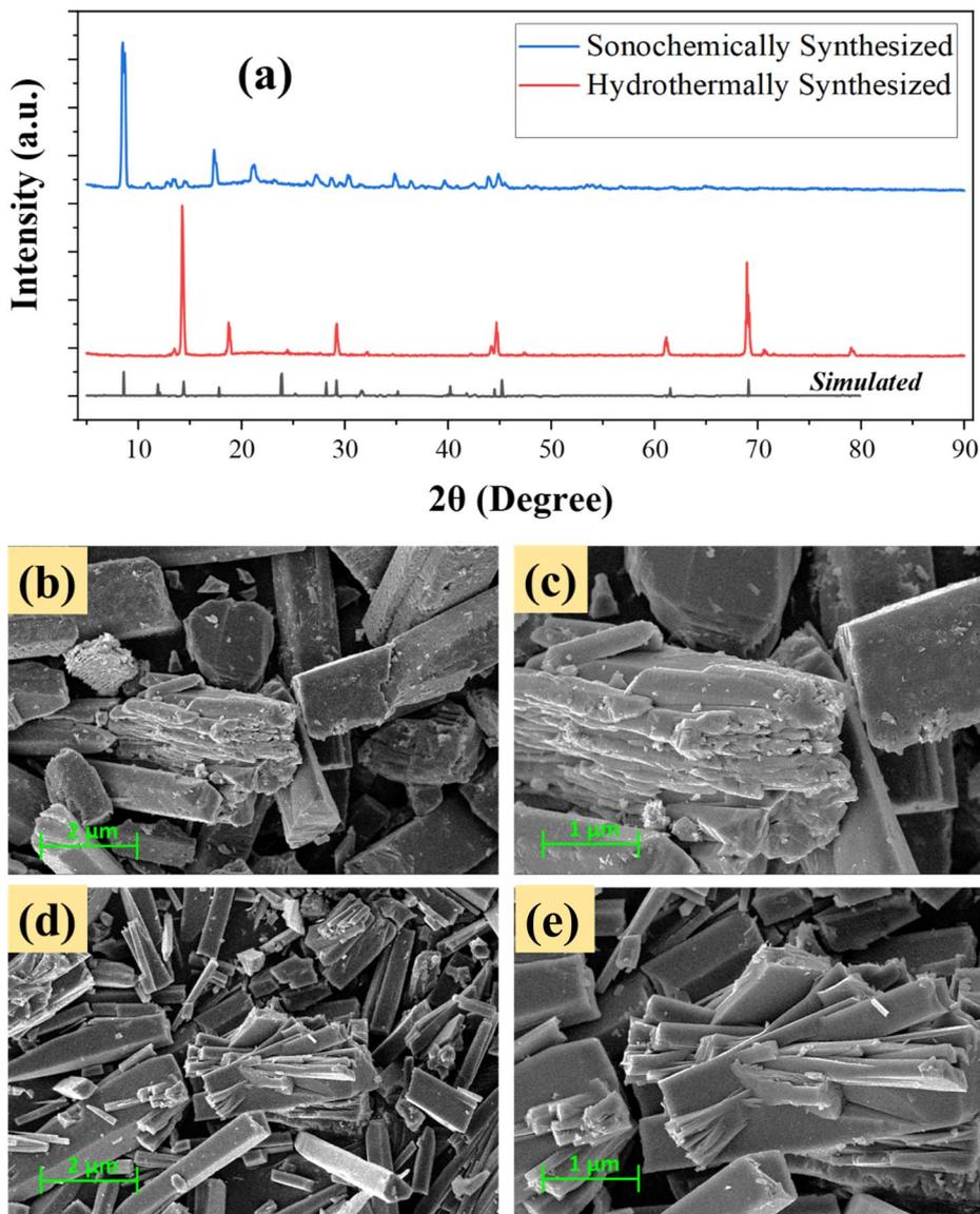
Fig. 2 (a) XRD analysis with multiple peaks demonstrating the crystallinity of Cu-MOF synthesized *via* the hydrothermal and sonochemical approach, respectively, (b and c) SEM results unveiling the morphology of Q1 and (d and e) for Q2.
