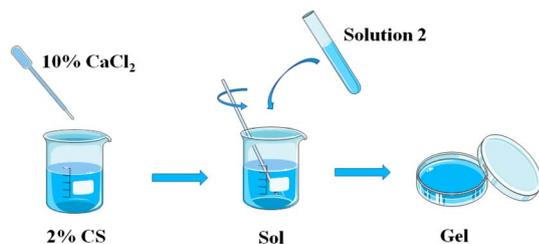
Fig. 1 Preparation process of the DP-CS-SA hydrogel.
