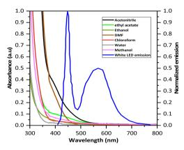
Fig. 1 Absorption spectra of NBS in different solvents at the reaction concentration and normalized emission spectra of used white LED.
