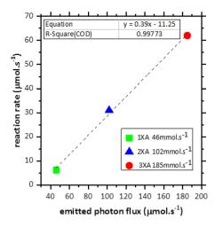
Fig. 4 Correlation graph of the reaction rate for the bromination reaction of 6-chloro-3-methyluracil with the reaction scale (left) and emitted photon flux (right) for the 1XA, 2XA and 4XA reactor modules at  $\Delta t = 0-900$  s.
