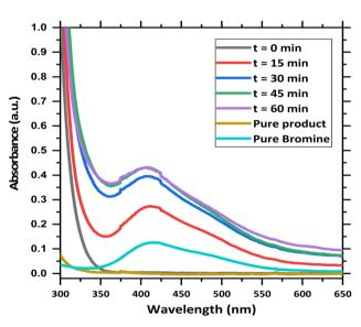
Fig. 2 Comparison of the absorbance data of the reaction mixture at different time intervals and pure product with respect to molecular bromine.
