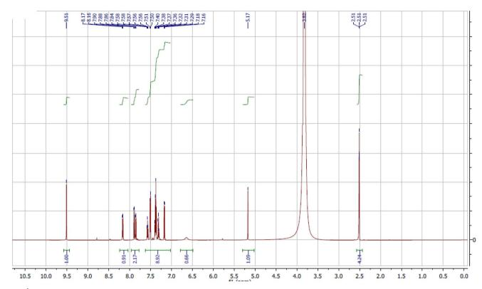
Fig. 2 <sup>1</sup>H-NMR spectrum of the ligand PANH in DMSO-d<sub>6</sub> solvent.
