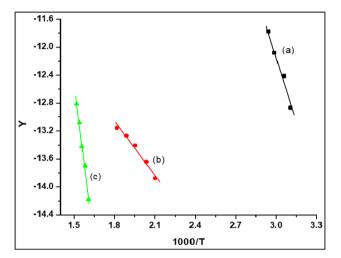
Fig. 7 Coats—Redfern plot for PANH-Mn (up) and PANH-Ni (down). (a) first step (b) second step (c) third step where,  $Y = [-\ln(1 - \alpha)]/T^2$  for n = 1.
