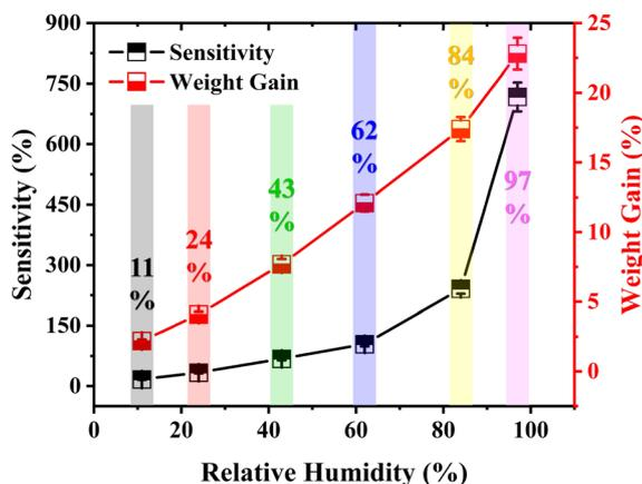
Fig. 4 Sensitivity and weight gain of the sensor in response to the increasing RH level.
