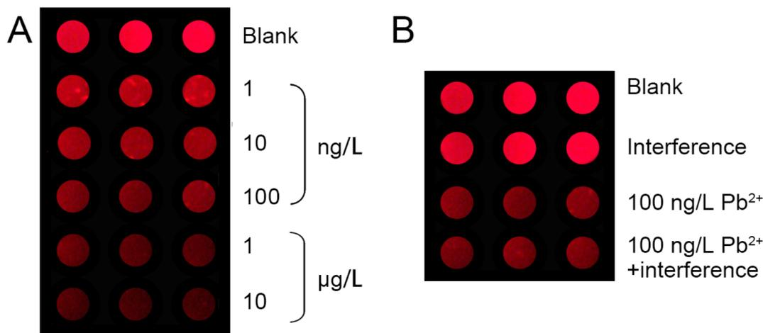
**Fig. 3** The visualization of Pb<sup>2+</sup> by the device. (A) The device response upon treatment with Pb<sup>2+</sup> solutions across varying concentrations, illustrating dose-dependent ECL intensity changes; (B) the selectivity assessment in the presence of different designated interfering ions, confirming minimal cross-reactivity. All scans were conducted at a rate of 400 mV s<sup>-1</sup>.
