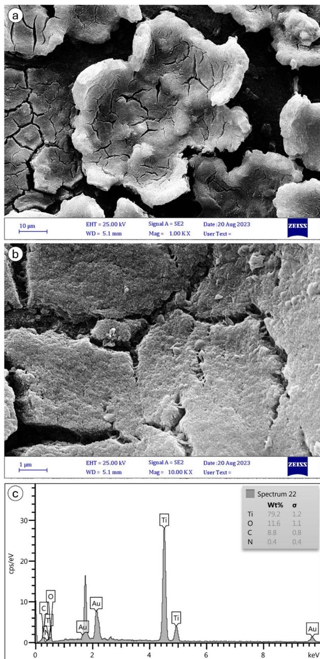
Fig. 7 SEM images of MIL-125 nanostructures of (a)  $\times 100$  k and (b)  $\times 10$  k magnifications, and (c) its EDAX spectrum.
