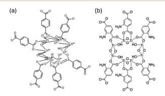
Fig. 1 The molecular structures of (a) MIL-125 and (b) NH<sub>2</sub>-MIL-125.
