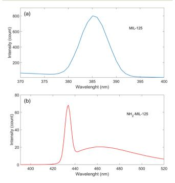
Fig. 6 PL spectra of (a) MIL-125 and (b)  $NH_2$ -MIL-125 nanostructures excited by high-intensity 345 nm and 429 nm beams, respectively.
