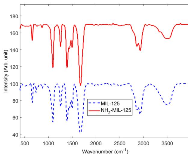
Fig. 2 FTIR spectra of MIL-125 and NH<sub>2</sub>-MIL-125.
