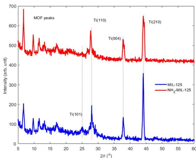
Fig. 5 XRD of MIL-125 and  $\text{NH}_2$ -MIL-125.
