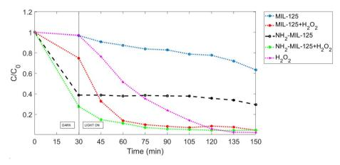
Fig. 10 The MB degradation with different photocatalytic conditions in UVC.
