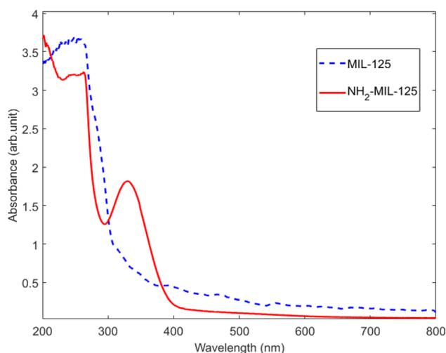
Fig. 3 UV-visible spectra of MIL-125 and  $\text{NH}_2\text{-MIL-125}$ .
