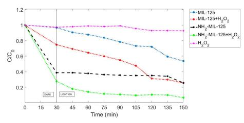
Fig. 11 The MB degradation with different photocatalytic conditions in visible.
