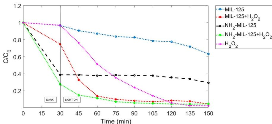
Fig. 10 The MB degradation with different photocatalytic conditions in UVC.
