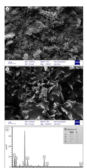
Fig. 8 SEM images of NH $_2$ -MIL-125 nanostructures of (a)  $\times 100$  k and (b)  $\times 10$  k magnifications, and (c) its EDAX spectrum.
