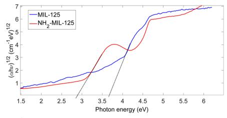
Fig. 4 Bandgap (plots of  $(\alpha \hbar n)^{1/2}$  versus the photon energy) of MIL-125 and NH<sub>2</sub>-MIL-125
