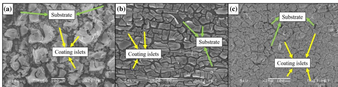
Fig. 6 SEM images of Ta<sub>2</sub>O<sub>5</sub>-coated AZ91 Mg alloy (a) C<sub>1</sub>, (b) C<sub>2</sub>, and (c) C<sub>3</sub> (Reproduced from ref. 45 with permission from Springer Nature copyright [2024]).
