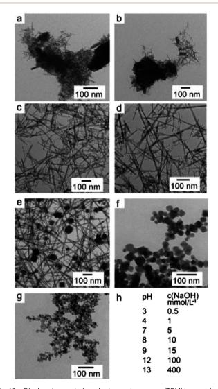
Fig. 10 Displays transmission electron microscopy (TEM) images (a-g) depicting tantalum oxide nanoparticles at various pH levels: (a) pH 3, (b) pH 4, (c) pH 7, (d) pH 8, (e) pH 9, (f) pH 12, and (g) pH 13. Additionally, (h) presents the pH values of the reaction mixtures prior to hydrothermal treatment, as determined by NaOH concentration (Reproduced from ref. 60 with permission from Royal Society of Chemistry copyright [2024]).
