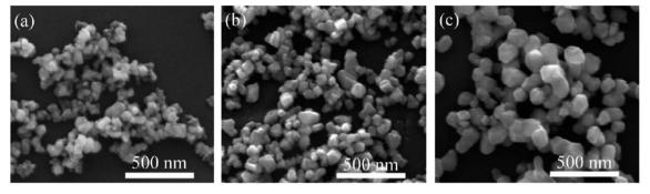
Fig. 8 FESEM images of powders synthesized at the C/Ta molar ratio of 4.25 at different temperatures: (a) 1400 °C, (b) 1500 °C, (c) 1600 °C (Reproduced from ref. 46 with permission from Elsevier copyright [2024]).
