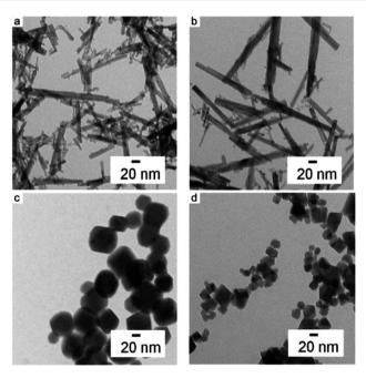
Fig. 11 TEM images of the nanoparticles yielded with different bases at different pH values. (a) pH 7 with KOH, (b) pH 7 with RbOH as the precursor base and (c) KOH and (d) RbOH as precursor bases both at pH 12 (Reproduced from ref. 60 with permission from Royal Society of Chemistry copyright [2024]).
