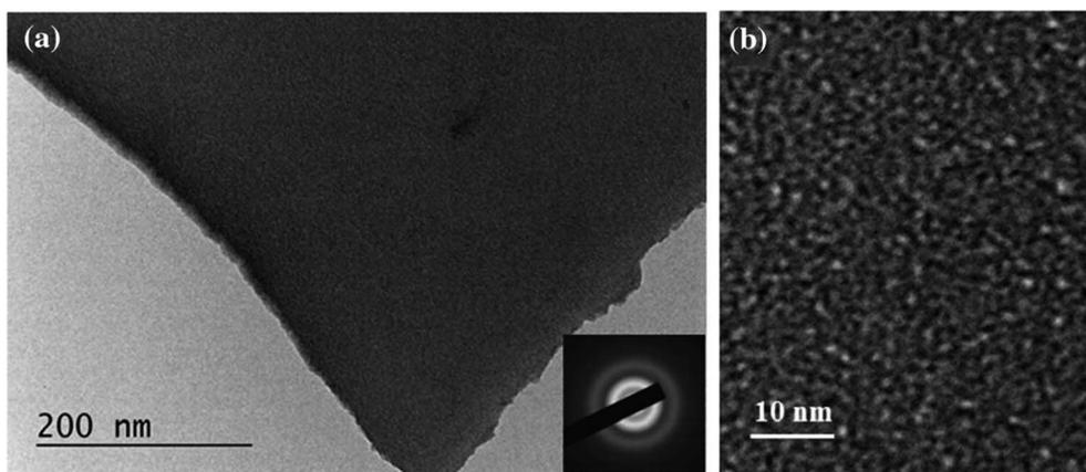
Fig. 1 TEM images and SAED pattern (inset) of dense Ta<sub>2</sub>O<sub>5</sub> films at different magnifications (a) 40 000× and (b) 150 000× (Reproduced from ref. 43 with permission from Springer Nature copyright [2024]).
