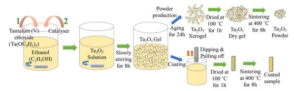
Fig. 5 Preparation of sol-gel solution and the steps for powder producing and coating processes (Reproduced from ref. 45 with permission from Springer Nature copyright [2024]).
