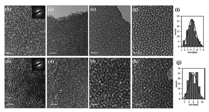
Fig. 2 TEM images of porous  $Ta_2O_5$  films prepared with addition of 5% organic template of copolymers PE6200 (a), PE6400 (c), PE6800 (e) and PE9400 (g) and 20% of PE6200 (b), PE6400 (d), PE6400 (f) and 15% of PE9400 (h); size distribution of the pores of  $Ta_2O_5$  templated with 5% PE9400 (i) and 15% PE9400 (j). (Inset): typical SAED (selected area electron diffraction) pattern. The bar is 20 nm (ref. 43) (Reproduced from ref. 43 with permission from Springer Nature copyright [2024]).
