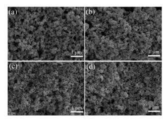
Fig. 7 SEM images of the powders prepared at different C/Ta molar ratios by SPS at 1500 °C for 5 min: (a) C/Ta = 3.75, (b) C/Ta = 4.00, (c) C/Ta = 4.25, (d) C/Ta = 4.50 (Reproduced from ref. 46 with permission from Elsevier copyright [2024]).
