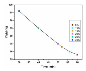
Fig. 5 Loading of IL (w/w%) on chitosan for the reaction of benzoic acid and ethanol catalysed by Chitosan-IL $_6$ .
