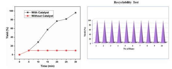
Fig. 6 (a) Hot filtration test to determine ionic liquid leaching of Chitosan-IL<sub>6</sub>. (b) Recyclability test of Chitosan-IL<sub>6</sub> catalyzed esterification of benzoic acid and ethanol to ethyl benzoate C1.
