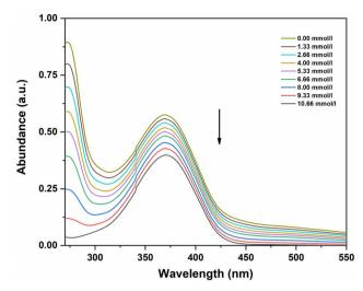
Fig. 4 UV-visible spectra of p-nitroaniline for various concentrations of ionic liquid ([BCPPD][Br]) in DMSO.
