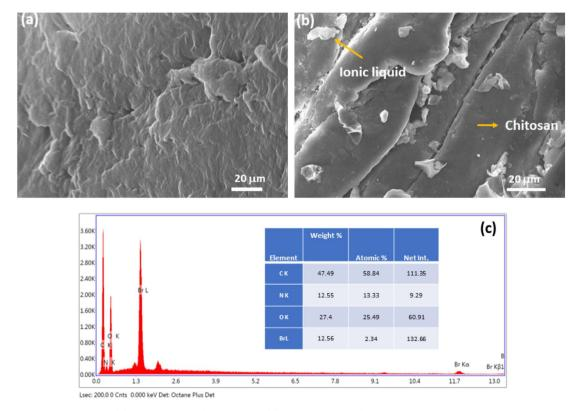
$\label{eq:Fig.3} \textbf{Fig. 3} \quad \textbf{(a) SEM image of Chitosan. (b) Sem image of Chitosan-IL}_{6}. \ \textbf{(c) EDX spectra of Chitosan-IL}_{6}.$
