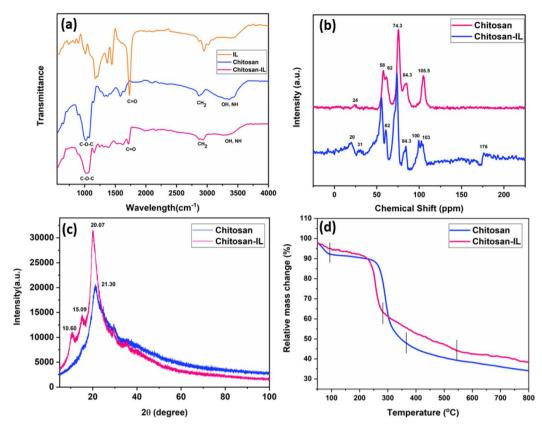
Fig. 2 (a) FT-IR spectra of IL<sub>6</sub>, chitosan and Chitosan-IL<sub>6</sub>. (b)  $^{13}$ C-CPMAS of chitosan and Chitosan-IL<sub>6</sub>. (c) PXRD of chitosan and Chitosan-IL<sub>6</sub>. (d) TGA of chitosan and Chitosan-IL<sub>6</sub>.
