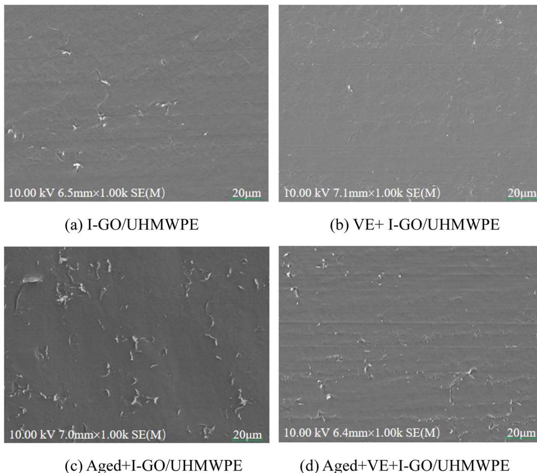
Fig. 8 SEM images of worn surface: I-GO/UHMWPE (a); VE+I-GO/UHMWPE (b); Aged+I-GO/UHMWPE (c); Aged+VE+I-GO/UHMWPE (d).
