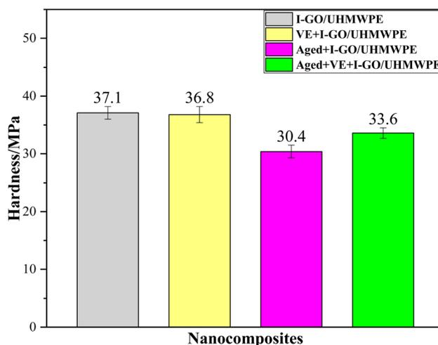
Fig. 6 Ball indentation hardness of the nanocomposites.
