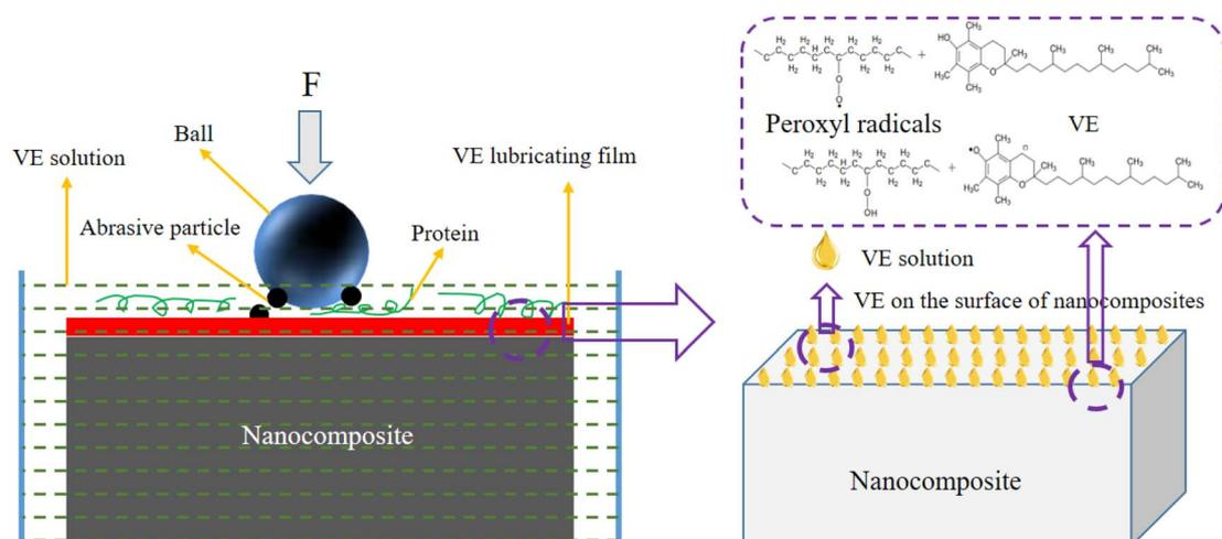
Fig. 9 Anti-friction and wear resistance mechanism of VE.
