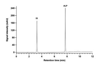
Fig. 2 Chromatogram of ALP and IS standard solutions at 50  $\mu g$  mL $^{-1}$ , detection at 315 nm.
