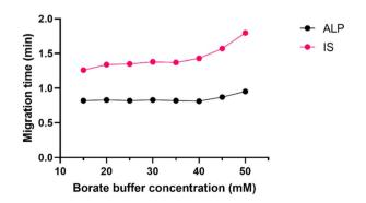
Fig. 3 Effect of borate buffer concentration (15–50 mM) on ALP and IS migration times, pH 9.3, 30  $^{\circ}$ C, 30 kV.
