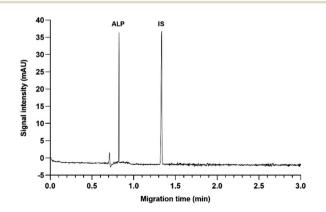
Fig. 1 CZE electropherogram of ALP and IS standard solutions at 50  $\mu g\ mL^{-1},$  25 mM borate at pH 9.3, 30 kV, 30 °C.
