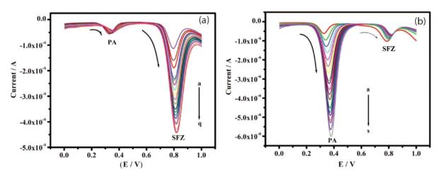
Fig. 6 (a) DPV profile of SUZ in the presence of 0.1 mM paracetamol at CdO/CPE. (b) Voltammogram of paracetamol in the presence of constant 0.1 mM SUZ using the same modified electrode. <sup>124</sup> Reproduced with permission from ref. 124. Copyright (2023) *Inorg. Chem. Commun.*
