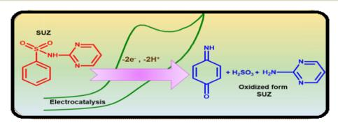
Scheme 2 Electro-oxidation mechanism of sulphadiazine drug at Cu<sub>2</sub>Sb/SPCE.<sup>122</sup>
