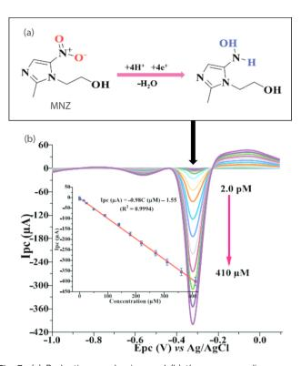
Fig. 7 (a) Reduction mechanism and (b) the corresponding square wave voltammogram of MNZ at TA-Au-Ag-ANpM/r-GO/poly(-glycine)/GCE within a potential range of -1.2 to 0.1 V, having reduction peak potential of -0.3 V. The inset shows a linear relationship between the reduction peak current and concentration of MNZ.<sup>133</sup> Reproduced with permission from ref. 133. Copyright (2024) *Chemosphere*.
