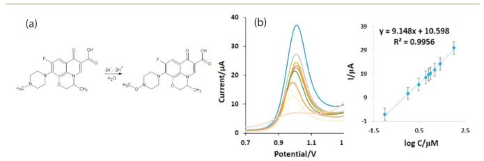
Fig. 8 (a) Mechanism of levofloxacin and (b) the DPV voltammogram at varying concentrations from 0.1 to 100 μM using AuNPs/rGO/GCE. Reproduced with permission from ref. 138. Copyright (2019) *Microchem. J.*<sup>138</sup>
