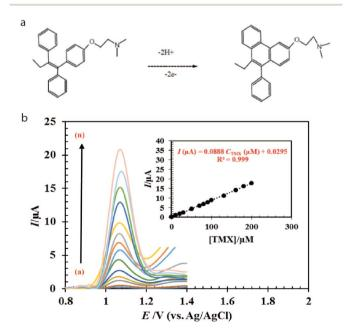
Fig. 2 (a) Oxidation mechanism of TMX and (b) its corresponding DPV signal recorded at  $Al_2O_3$ @C/ $V_2O_5$ /CPE (inset, represents the linear range of 0.1 to 200  $\mu$ M under optimized conditions. <sup>68</sup> Reproduced with permission from ref. 68. Copyright (2022) *Microchem. J.*
