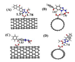
**Fig. 10** The optimized configuration of MBZ on functionalized CNTs is represented by (A), (B), (C), (D) and bond distance expressed in angstrom. <sup>94</sup> Reproduced with permission from ref. 94. Copyright (2016) *Mater. Sci. Eng.*
