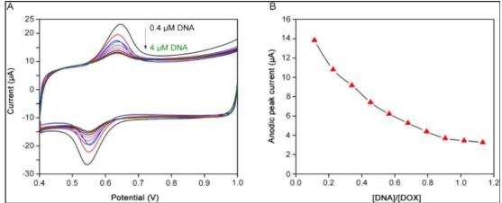
Fig. 4 (A) CV profile of DOX at MWCNTs/Pt electrode following the successive insertion of DNA. (B) and the corresponding reduction of peak current confirming the Drug – DNA adduct.<sup>90</sup>
