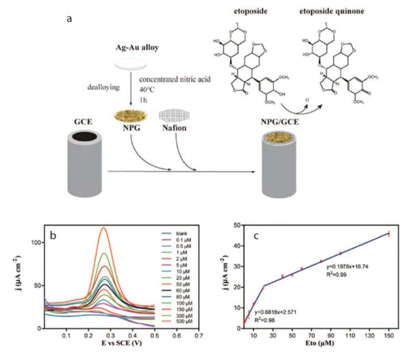
Fig. 3 (a) Shows the fabrication of the sensor (NPG/GCE) and (b) corresponding DPV profile of ETO at an oxidation peak potential of  $0.3\,V$  (c) with two linear ranges of  $0.1-20\,\mu\text{M}$  and  $20-150\,\mu\text{M}$ .
