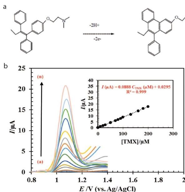
Fig. 2 (a) Oxidation mechanism of TMX and (b) its corresponding DPV signal recorded at Al<sub>2</sub>O<sub>3</sub>@C/V<sub>2</sub>O<sub>5</sub>/CPE (inset, represents the linear range of 0.1 to 200  $\mu\text{M}$  under optimized conditions.<sup>68</sup> Reproduced with permission from ref. 68. Copyright (2022) *Microchem. J.*
