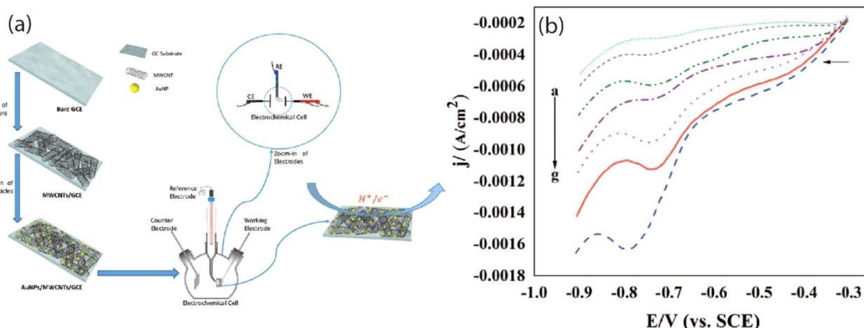
Fig. 5 (a) Fabrication of MWCNTs-COOH/AuNPs/GCP and (b) corresponding LSV response of reduction of  $5 \mu\text{M}$  DOX in  $0.1$  M PBS of pH  $7$ .<sup>82</sup>
