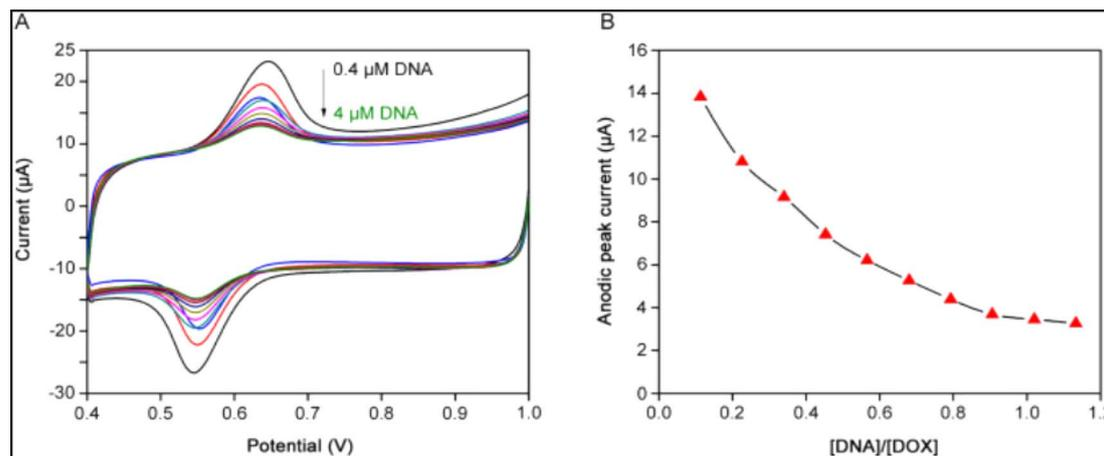
Fig. 4 (A) CV profile of DOX at MWCNTs/Pt electrode following the successive insertion of DNA. (B) and the corresponding reduction of peak current confirming the Drug – DNA adduct.<sup>80</sup>
