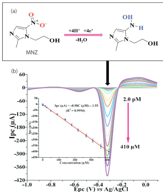
Fig. 7 (a) Reduction mechanism and (b) the corresponding square wave voltammogram of MNZ at TA-Au-Ag-ANpM/r-GO/poly(glycine)/GCE within a potential range of  $-1.2$  to  $0.1$  V, having reduction peak potential of  $-0.3$  V. The inset shows a linear relationship between the reduction peak current and concentration of MNZ.<sup>133</sup> Reproduced with permission from ref. 133. Copyright (2024) *Chemosphere*.
