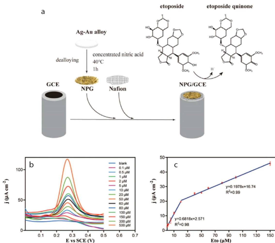
Fig. 3 (a) Shows the fabrication of the sensor (NPG/GCE) and (b) corresponding DPV profile of ETO at an oxidation peak potential of 0.3 V (c) with two linear ranges of 0.1–20  $\mu$ M and 20–150  $\mu$ M.<sup>106</sup>
