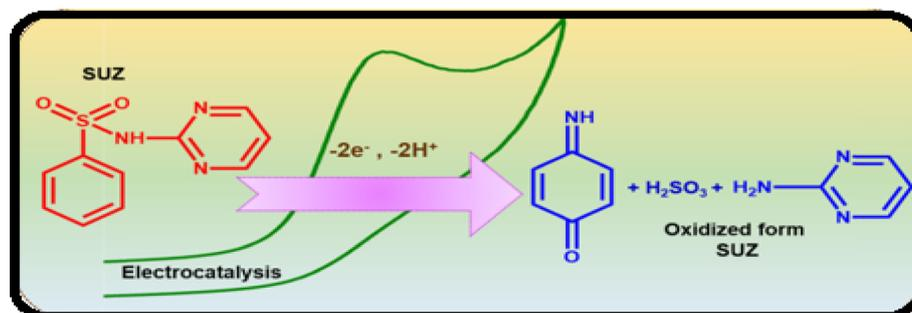
Scheme 2 Electro-oxidation mechanism of sulphadiazine drug at Cu<sub>2</sub>Sb/SPCE.<sup>122</sup>
