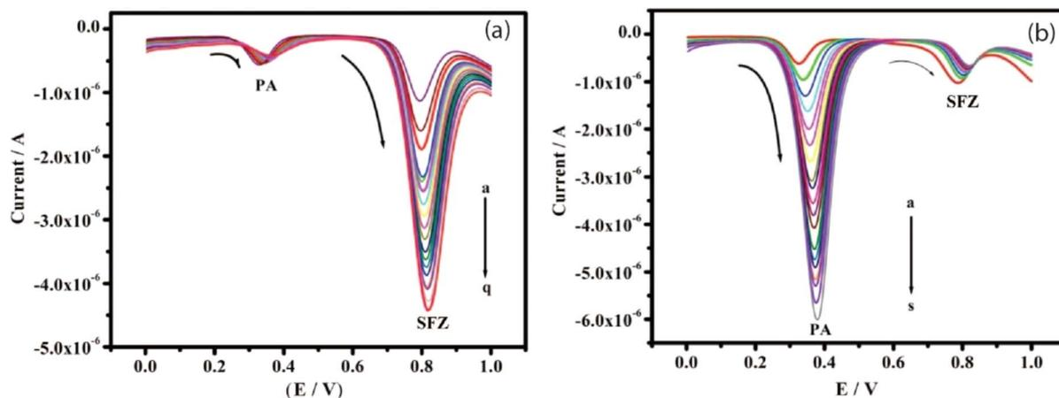
Fig. 6 (a) DPV profile of SUZ in the presence of 0.1 mM paracetamol at CdO/CPE. (b) Voltammogram of paracetamol in the presence of constant 0.1 mM SUZ using the same modified electrode.<sup>124</sup> Reproduced with permission from ref. 124. Copyright (2023) *Inorg. Chem. Commun.*
