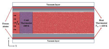
Fig. 1 Schematic diagram of the MD simulation system for convection.
