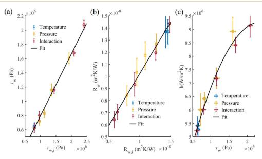
Fig. 11 (a) Wall shear stress obtained by eqn (7) and (9), (b) interfacial thermal resistance obtained by eqn (4) and (5), (c) convective heat transfer coefficient as a function of wall shear stress under different water temperature ( $\varepsilon = 0.003992$  eV, P = 1 bar), pressures ( $T_{in} = 280$  K,  $\varepsilon = 0.003992$ eV) and interaction strengths ( $T_{in} = 280 \text{ K}$ , P = 1 bar).
