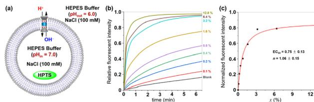
Fig. 4 (a) Schematic representation for the HPTS assay. (b) Changes in the relative fluorescence intensity of HPTS ( $\lambda_{\text{ex}} = 460 \text{ nm}$ ,  $\lambda_{\text{em}} = 510 \text{ nm}$ ) in vesicles with time in the presence of varying concentrations of **1** (molar ratio relative to lipid, represented by  $x$ ). (c) Changes in normalized fluorescent intensity of HPTS in vesicles with the concentration of **1**. Curve-fitting analyses were carried out by the Hill equation.
