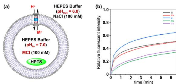
Fig. 6 (a) Schematic representation for the HPTS assay with varied internal metal ions ( $M^+ = \text{Li}^+, \text{Na}^+, \text{K}^+, \text{Rb}^+$  and  $\text{Cs}^+$ ). (b) Changes in the fluorescence intensity of cation transport activity test of **1** ( $x = 0.8\%$ ).
