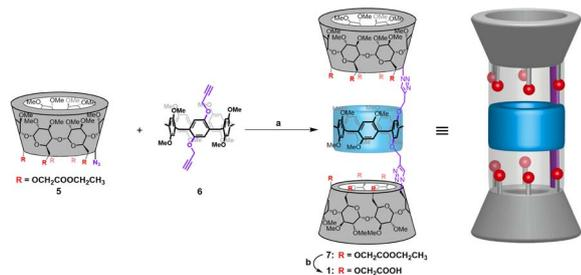
Fig. 2 Synthesis and structural features of channel 1: (a)  $\text{CuSO}_4 \cdot 5\text{H}_2\text{O}$ , sodium ascorbate, DMSO, r.t.; (b)  $\text{LiOH} \cdot \text{H}_2\text{O}$ ,  $\text{MeOH}/\text{H}_2\text{O}$ , r.t.
