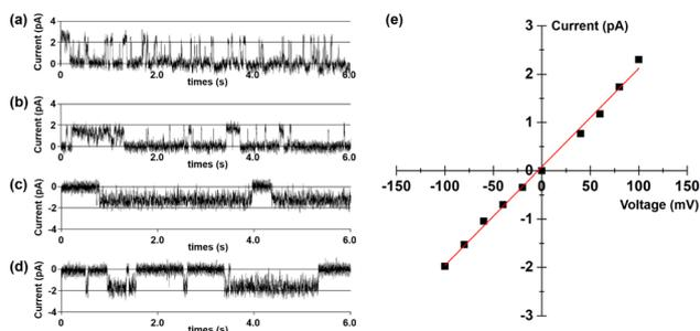
Fig. 8 Current traces through a planar lipid bilayer in 1.0 M KCl at a potential of (a) +100 mV, (b) +80 mV, (c) -80 mV and (d) -100 mV in the presence of **1**. (e)  $I$ - $V$  curve of **1** (0.25  $\mu\text{M}$ ) in the planar lipid bilayer in a symmetrical 1.0 M KCl solution.
