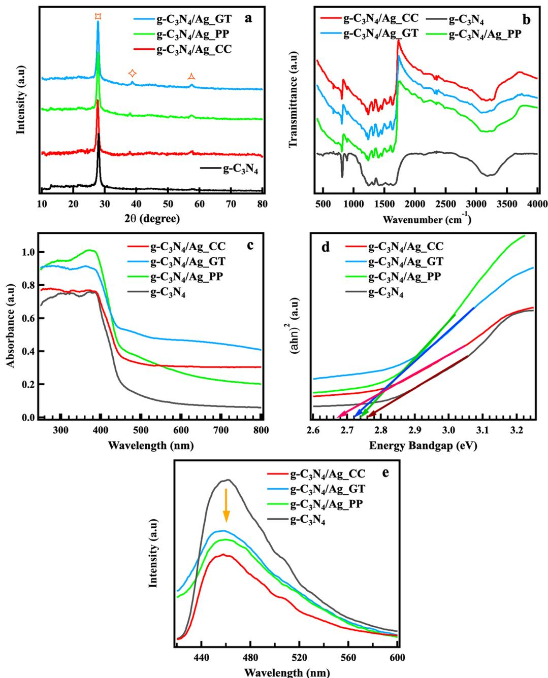
Fig. 4 XRD patterns (a), FTIR spectra (b), UV-vis DRS spectra (c), Tauc plot (d), PL spectra (e) of  $g\text{-C}_3\text{N}_4$ ,  $g\text{-C}_3\text{N}_4/\text{Ag}_{\text{CC}}$ ,  $g\text{-C}_3\text{N}_4/\text{Ag}_{\text{GT}}$ ,  $g\text{-C}_3\text{N}_4/\text{Ag}_{\text{PP}}$ .
