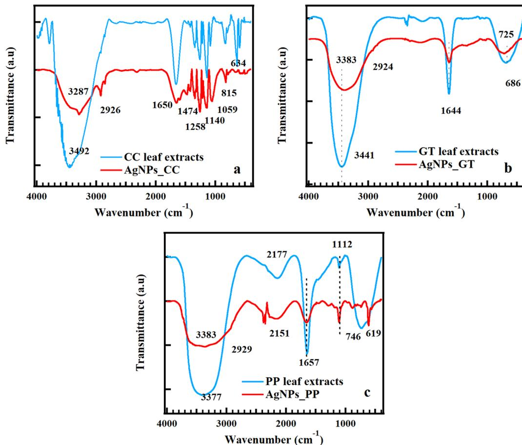
Fig. 3 FTIR spectra of CC leaf extract and AgNPs<sub>CC</sub> (a), GT leaf extract and AgNPs<sub>GT</sub> (b), PP leaf extract and AgNPs<sub>PP</sub> (c).
