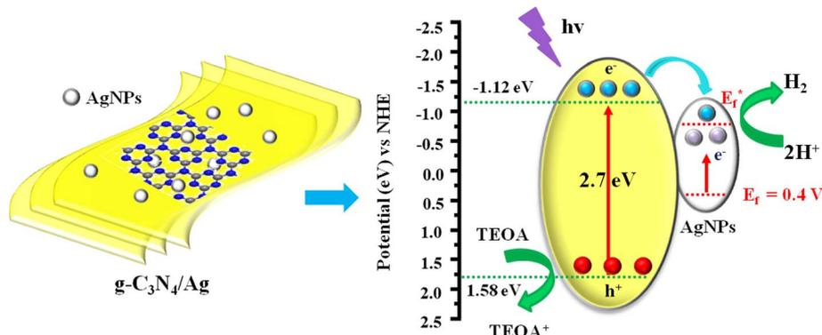
Fig. 8 Proposal mechanism for PH2P of g-C<sub>3</sub>N<sub>4</sub>/Ag.
