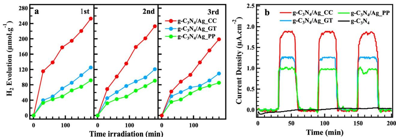
Fig. 7 Photocatalytic hydrogen production in three consecutive cycles (a), transient photocurrent (b) of  $g\text{-C}_3\text{N}_4/\text{Ag\_CC}$ ,  $g\text{-C}_3\text{N}_4/\text{Ag\_GT}$ ,  $g\text{-C}_3\text{N}_4/\text{Ag\_PP}$ , and  $g\text{-C}_3\text{N}_4$  under visible-light irradiation.
