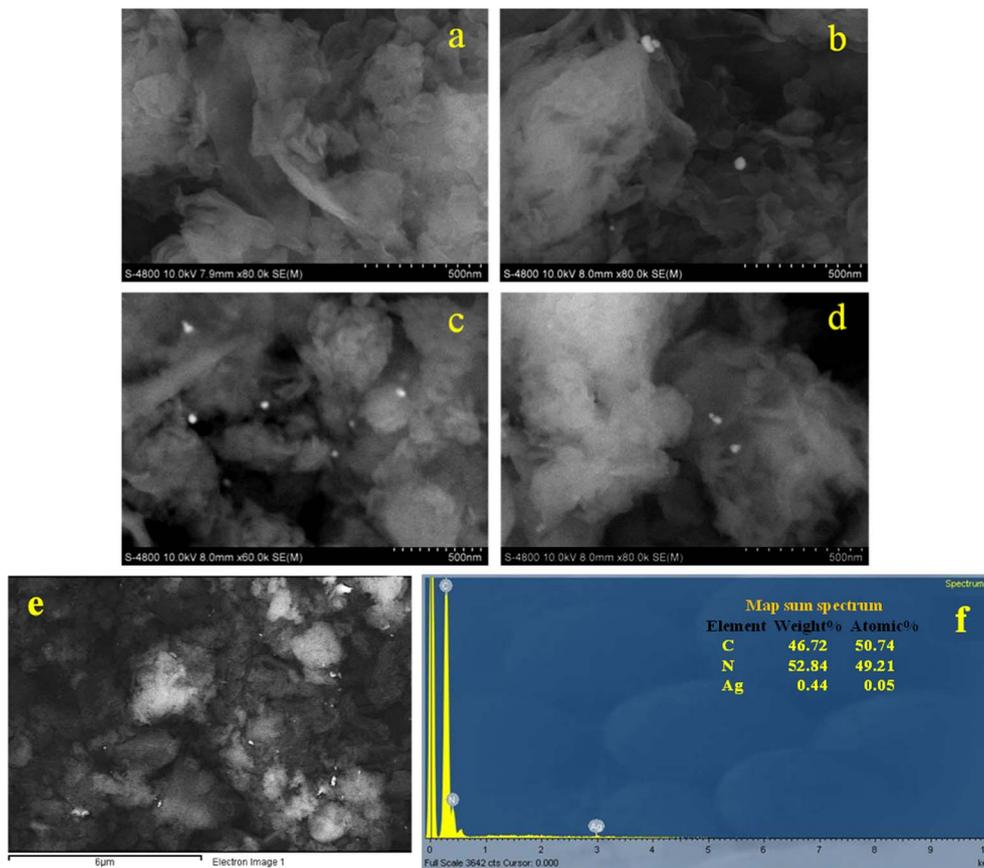
Fig. 5 SEM images of  $g\text{-C}_3\text{N}_4$  (a),  $g\text{-C}_3\text{N}_4/\text{Ag\_CC}$  (b),  $g\text{-C}_3\text{N}_4/\text{Ag\_GT}$  (c), and  $g\text{-C}_3\text{N}_4/\text{Ag\_PP}$  (d), EDX analysis of  $g\text{-C}_3\text{N}_4/\text{Ag\_CC}$  (e and f).
