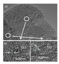
Fig. 3 (a) TEM of the MS-400 nanocatalyst, and HRTEM of (b)  $MoO_3$  and (c)  $MoS_2$ .
