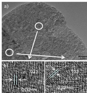
Fig. 3 (a) TEM of the MS-400 nanocatalyst, and HRTEM of (b) MoO<sub>3</sub> and (c) MoS<sub>2</sub>.
