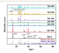
Fig. 1 XRD patterns of the samples.
