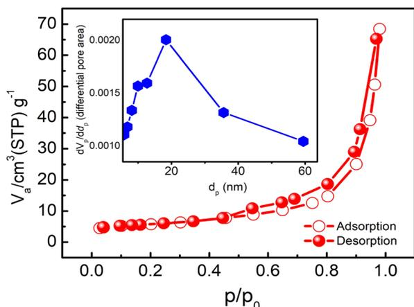
Fig. 6 Nitrogen adsorption–desorption isotherm at 77 K and pore size distribution (inset) for the as prepared  $\delta$ -MnO<sub>2</sub> nanoflowers.
