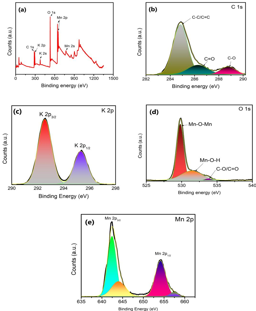
Fig. 4 (a) XPS survey spectra for  $\delta$ -MnO<sub>2</sub> nanoflowers and fitting corresponding to (b) C, (c) K, (d) O and (e) Mn elements.
