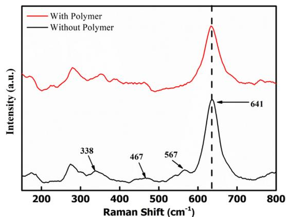
Fig. 5 Raman spectra for  $\delta$ -MnO<sub>2</sub> nanoflowers with and without a polymer.
