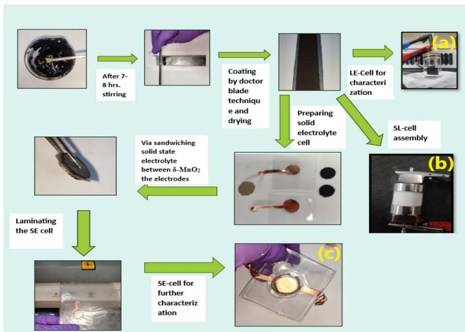
Fig. 1 Process for making  $\delta$ -MnO<sub>2</sub>-nanoflower-polymer electrodes and supercapacitors. Abbreviations: LE-cells: liquid electrolyte based cells in a 3-electrode setup, SL-cells: supercapacitors assembled in a Swagelok 2-electrode geometry, and SE-cells: all-solid-state supercapacitors assembled in a 2-electrode geometry.
