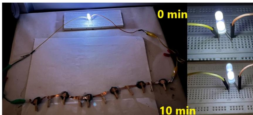
**Fig. 10** LEDs each of 3 V ( $\sim 60 \text{ mW}$ ) during the direct discharge of SL cells for 10 minutes.
