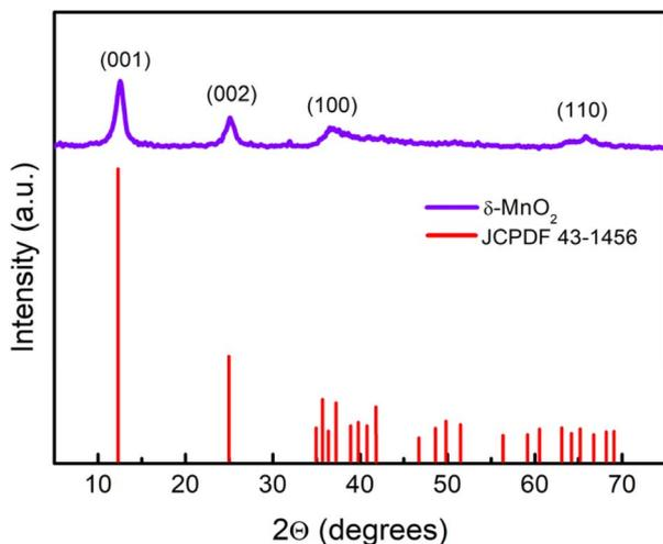
Fig. 3 XRD pattern identified as the  $\delta$ -MnO<sub>2</sub> layered structure as per JCPDF card no. 43-1456. The crystallite size was calculated using the Scherrer formula  $\left(\frac{0.91\lambda}{\beta \cos \theta}\right)$ , where  $\lambda$ ,  $\theta$ , and  $\beta$  represent the X-ray wavelength, Bragg's angle and FWHM of the peak.
