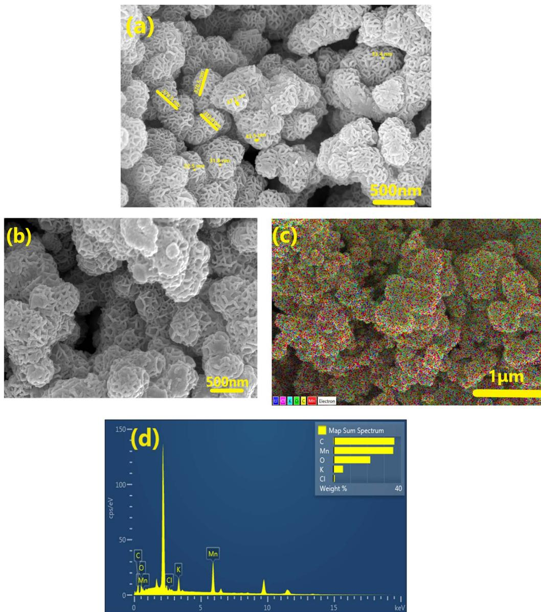
Fig. 2 FESEM investigations of (a) pristine  $\delta$ -MnO<sub>2</sub> nanoflowers and (b) MNF-polymer electrodes and (c) EDX with color spectrum and (d) EDS spectrum of MNF-polymer electrodes at 1  $\mu$ m.
