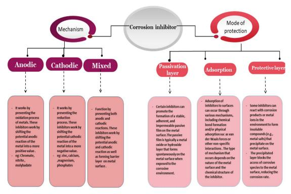
Fig. 3 Scheme of corrosion inhibitor role
