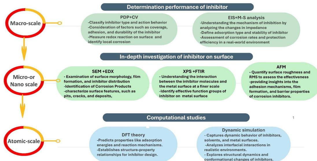
Fig. 10 Summary of inhibition performance validation approaches.
