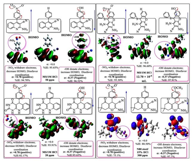
Fig. 4 Adsorption and coordination bonding behavior of pyridine, triazine and quinoline and their mono- and di-substituted derivative.<sup>134</sup>
