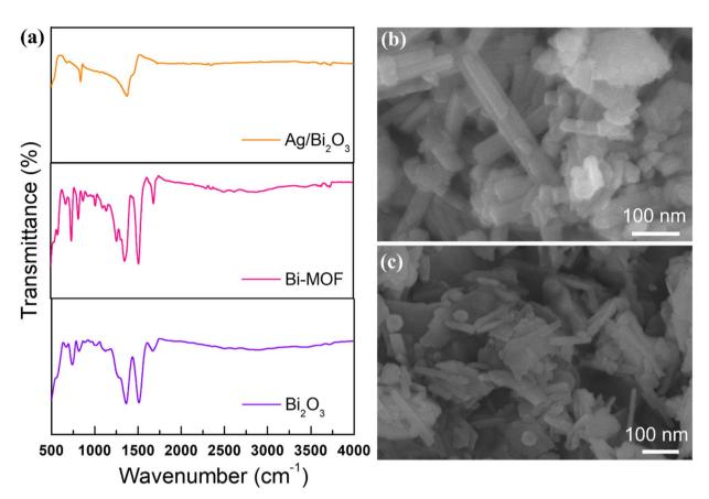
Fig. 7 (a) FTIR spectra of Bi-MOF,  $Bi_2O_3$ , and  $Ag/Bi_2O_3$  after the adsorption and photocatalysis process, (b) SEM images of Bi-MOF and (c)  $Ag/Bi_2O_3$  after the photocatalysis process.
