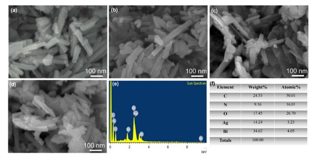
Fig. 3 SEM images of (a) Bi-MOF, (b)  $Bi_2O_3$ , (c) Ag/Bi-MOF, (d) Ag/Bi $_2O_3$ , (e) EDX spectrum of the Ag/Bi-MOF sample, (f) elemental weight% and atomic% distribution table of the Ag/Bi-MOF sample.
