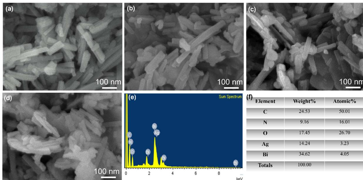
Fig. 3 SEM images of (a) Bi-MOF, (b)  $\text{Bi}_2\text{O}_3$ , (c) Ag/Bi-MOF, (d) Ag/ $\text{Bi}_2\text{O}_3$ , (e) EDX spectrum of the Ag/Bi-MOF sample, (f) elemental weight% and atomic% distribution table of the Ag/Bi-MOF sample.
