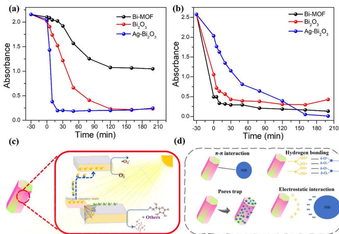
Fig. 5 (a) Synthesis, UV-vis absorption, and photocatalysis of Bi-MOF,  $\text{Bi}_2\text{O}_3$ , and  $\text{Ag}/\text{Bi}_2\text{O}_3$  for the removal of Rhodamine B (RhB); (b) UV-vis absorption and photocatalysis of Bi-MOF,  $\text{Bi}_2\text{O}_3$ , and  $\text{Ag}/\text{Bi}_2\text{O}_3$  for the removal of Methylene Blue (MB); (c) proposed mechanism of photocatalysis by Bi-MOF derivatives under visible light; (d) four possible adsorption mechanisms of Methylene Blue with Bi-MOF.
