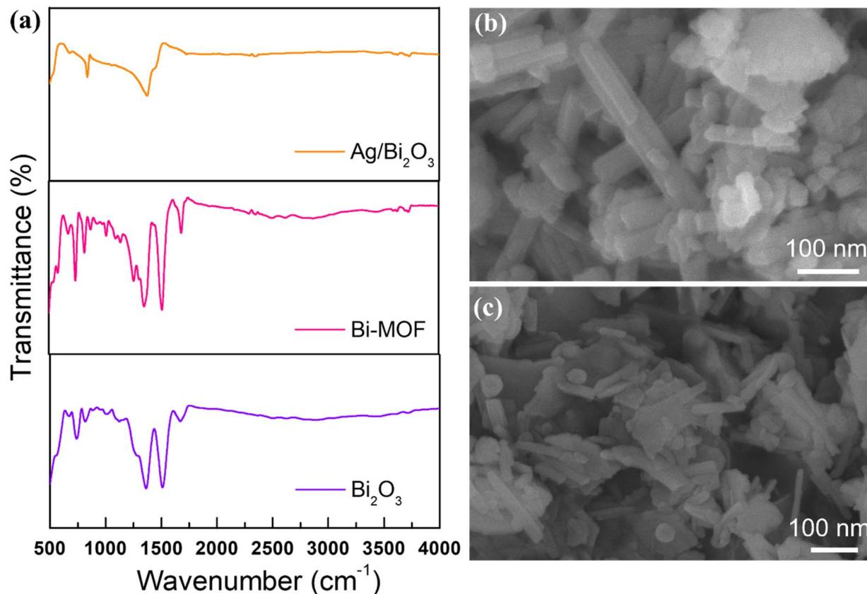
Fig. 7 (a) FTIR spectra of Bi-MOF,  $\text{Bi}_2\text{O}_3$ , and  $\text{Ag}/\text{Bi}_2\text{O}_3$  after the adsorption and photocatalysis process, (b) SEM images of Bi-MOF and (c)  $\text{Ag}/\text{Bi}_2\text{O}_3$  after the photocatalysis process.
