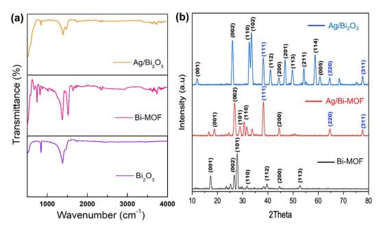
Fig. 1 (a) FTIR spectra of Bi-MOF, Bi<sub>2</sub>O<sub>3</sub>, and Ag/Bi<sub>2</sub>O<sub>3</sub>, (b) XRD spectra of Bi-MOF, Ag/Bi-MOF, and Ag/Bi<sub>2</sub>O<sub>3</sub>
