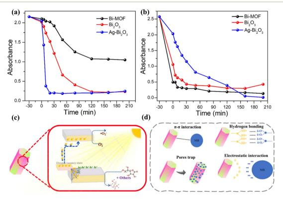
Fig. 5 (a) Synthesis, UV-vis absorption, and photocatalysis of Bi-MOF,  $Bi_2O_3$ , and  $Ag/Bi_2O_3$  for the removal of Rhodamine B (RhB); (b) UV-vis absorption and photocatalysis of Bi-MOF,  $Bi_2O_3$ , and  $Ag/Bi_2O_3$  for the removal of Methylene Blue (MB); (c) proposed mechanism of photocatalysis by Bi-MOF derivatives under visible light; (d) four possible adsorption mechanisms of Methylene Blue with Bi-MOF.
