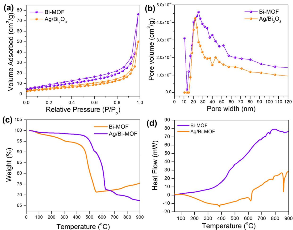
Fig. 2 (a) Nitrogen adsorption–desorption isotherm of Bi-MOF, Ag/Bi<sub>2</sub>O<sub>3</sub>, (b) pore size distribution of Bi-MOF, Ag/Bi<sub>2</sub>O<sub>3</sub>, (c) thermogravimetric analysis (TGA) and (d) differential scanning calorimetry (DSC) of Bi-MOF, Ag/Bi-MOF in the atmosphere.
