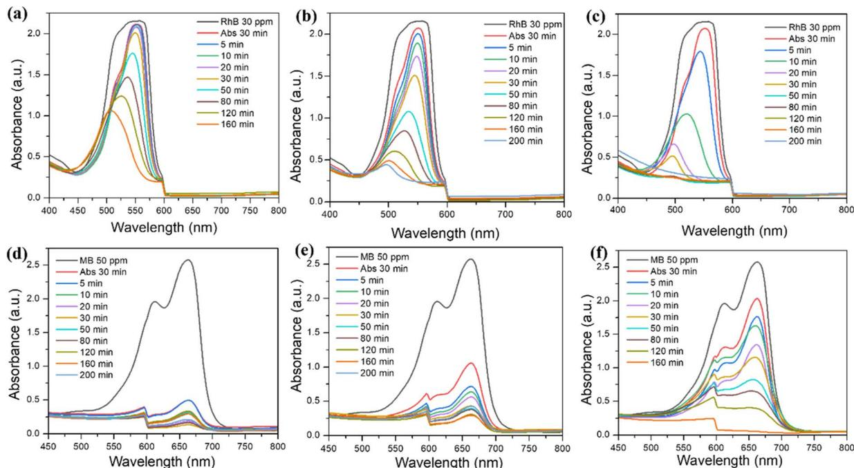
Fig. 4 UV-vis absorption and photocatalysis of (a) Bi-MOF, (b)  $\text{Bi}_2\text{O}_3$ , and (c)  $\text{Ag}/\text{Bi}_2\text{O}_3$  for the removal of Rhodamine B (RhB); UV-vis absorption and photocatalysis of (d) Bi-MOF, (e)  $\text{Bi}_2\text{O}_3$ , and (f)  $\text{Ag}/\text{Bi}_2\text{O}_3$  for the removal of Methylene Blue (MB).
