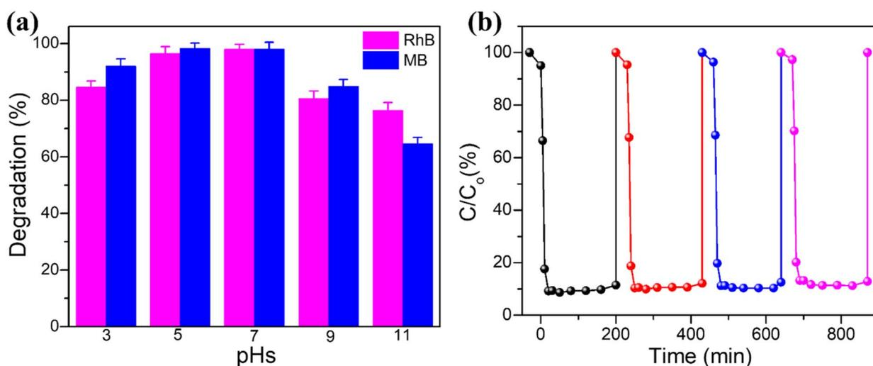
Fig. 6 (a) The influence of different pH values (3, 5, 7, 9, 11) on the degradation efficiency of RhB and MB by Ag/Bi<sub>2</sub>O<sub>3</sub>; (b) recycling performance of RhB degradation by Ag/Bi<sub>2</sub>O<sub>3</sub> after 4 cycles.
