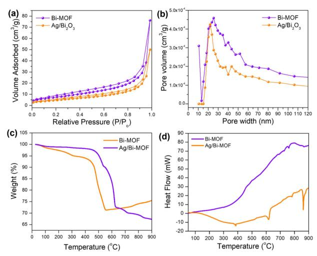
Fig. 2 (a) Nitrogen adsorption-desorption isotherm of Bi-MOF, Ag/Bi<sub>2</sub>O<sub>3</sub>, (b) pore size distribution of Bi-MOF, Ag/Bi<sub>2</sub>O<sub>3</sub>, (c) thermogravimetric analysis (TGA) and (d) differential scanning calorimetry (DSC) of Bi-MOF, Ag/Bi-MOF in the atmosphere.
