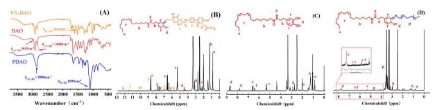
(A) Infrared spectra of PDAO, DAO and FA-DAO. NMR hydrogen spectra of (B) FA-DAO, (C) DAO and (D) PDAO.
