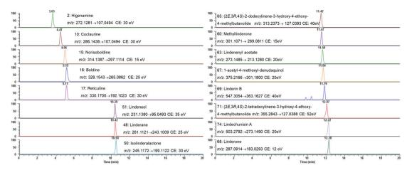
Fig. 2 Extracted ion chromatograms of the quantified analytes in PRM mode.
