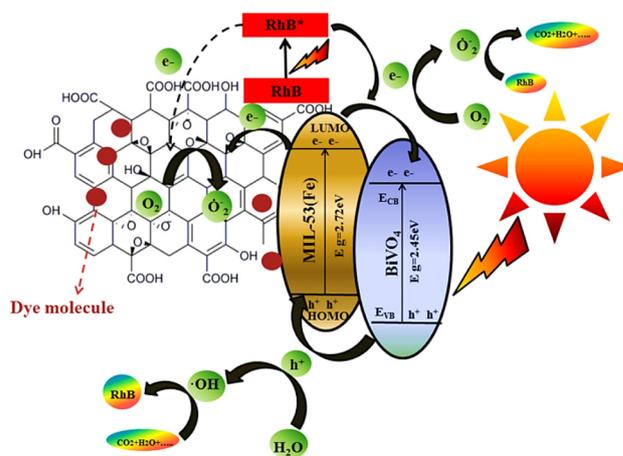
Fig. 17 Degradation of Rhodamine B (RhB) dye using BiVO<sub>4</sub>/MOF/GO nanocomposites. Reproduced with permission from ref. 159. Copyright (2020) Elsevier.
