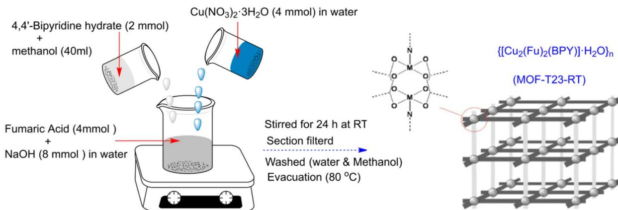
Fig. 8 Synthesis of the pillared-layer MOF,  $\{[Cu_2(Fu)_2(BPY)] \cdot H_2O\}_n$  via a chemical process.<sup>65</sup> Reproduced with permission from ref. 65 Copyright (2022) RCS Advances.
