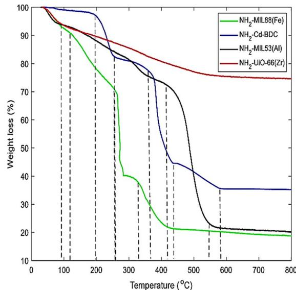
Fig. 14 Thermogravimetric analysis (TGA) of four MOFs:  $NH_2$ -UiO-66(Zr),  $NH_2$ -MIL53(Al),  $NH_2$ -Cd-BDC, and  $NH_2$ -MIL88(Fe). Reprinted with permission from ref. 90. Copyright (2022) Springer.
