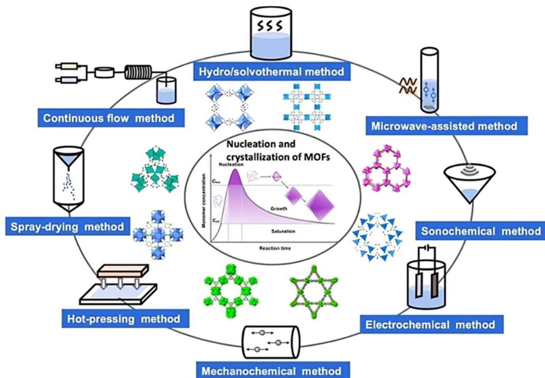
Fig. 2 Representation of the synthetic scheme of metal organic frameworks. Reproduced with access provided by HEC.<sup>34</sup>
