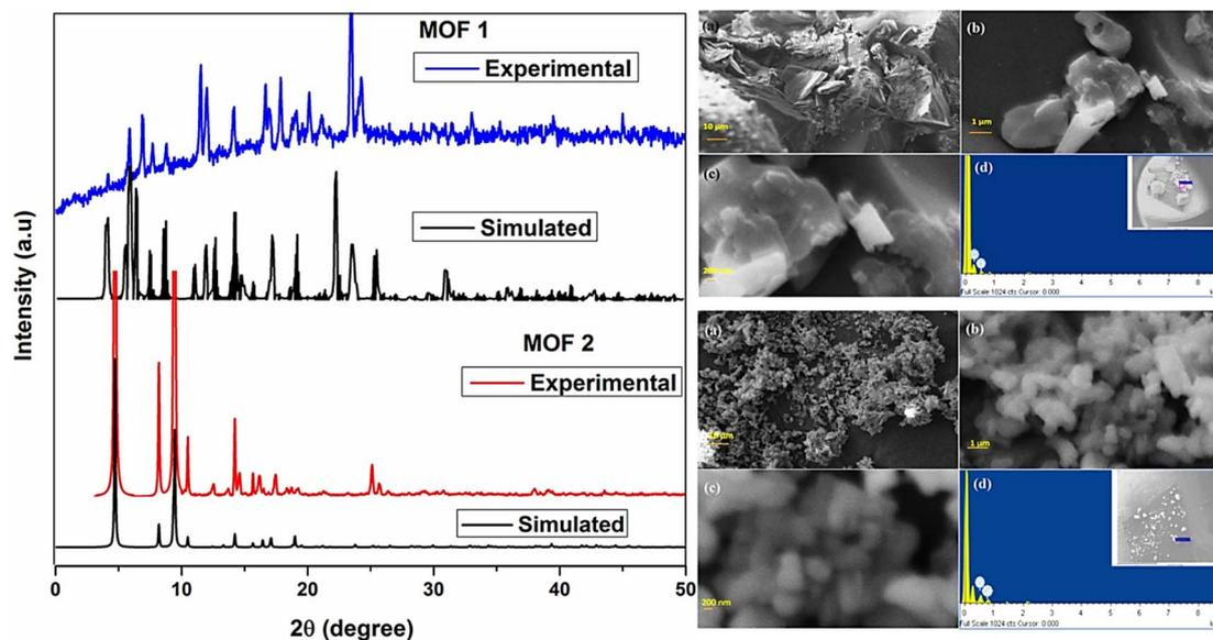
Fig. 11 Left: XRD spectra of mixed-ligand  $[\text{Co}(\text{BDC})(\text{Phen})(\text{H}_2\text{O})](1)$  and  $[\text{Co}(\text{BDC})(\text{DABCO})](2)$  MOFs. Top right (a–d): SEM-EDX analysis of mixed-ligand  $[\text{Co}(\text{BDC})(\text{Phen})(\text{H}_2\text{O})](1)$  MOF. Bottom right (a–d): SEM-EDX analysis of mixed-ligand  $[\text{Co}(\text{BDC})(\text{DABCO})](2)$  MOF. Reprinted with permission from ref. 80. Copyright (2021) Springer.
