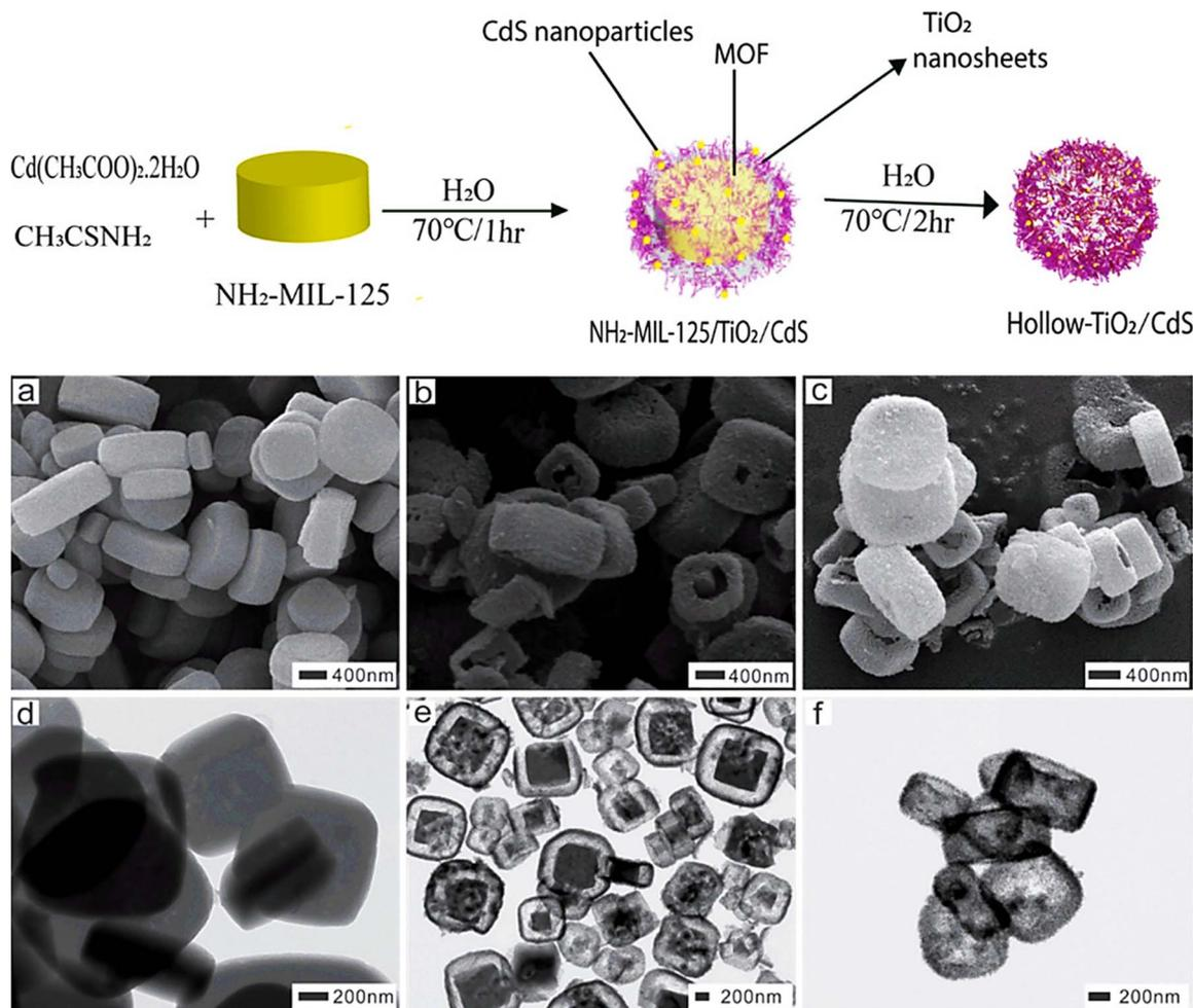
Fig. 5 Synthesis of  $\text{NH}_2\text{-MIL-125}/\text{TiO}_2/\text{CdS}$  yolk-shell and hollow  $\text{H-TiO}_2/\text{CdS}$  heterostructures. SEM (a–c) and TEM (d–f) images of  $\text{NH}_2\text{-MIL-125}$  MOF,  $\text{NH}_2\text{-MIL-125}/\text{TiO}_2/\text{CdS}$  yolk-shell, and  $\text{H-TiO}_2/\text{CdS}$ . Reproduced with permission from ref. 48. Copyright (2018) American Chemical Society.
