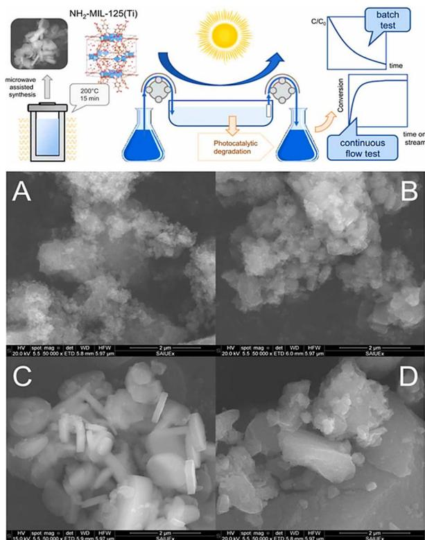
Fig. 6 Schematic of the microwave-assisted synthesis of  $\text{NH}_2\text{-MIL-125(Ti)}$  samples at different temperatures and periods, and SEM images of the samples: (A) 140 °C for 15 minutes; (B) 160 °C for 15 minutes; (C) 200 °C for 15 minutes; and (D) 200 °C for 4 hours. Reprinted with permission from ref. 55. Copyright (2021) Elsevier.
