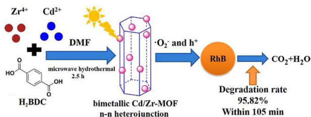
Fig. 3 Synthetic and photocatalytic activity of synthesized Cd/Zr-MOF nanomaterials. Reproduced with access provided by Higher Education Commission (HEC). 41
