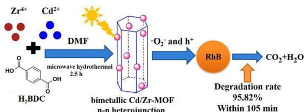
Fig. 3 Synthetic and photocatalytic activity of synthesized Cd/Zr-MOF nanomaterials. Reproduced with access provided by Higher Education Commission (HEC).<sup>41</sup>
