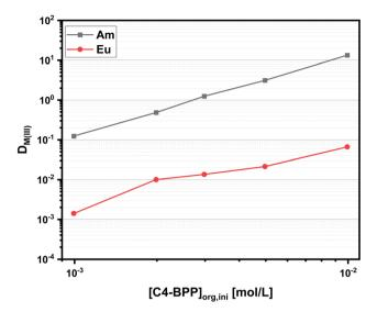
Fig. 4 Distribution ratios for the extraction of Am(III) and Eu(III) with C4-BPP. Organic phase 1.0  $\times$   $10^{-3}$ –1.0  $\times$   $10^{-2}$  mol L $^{-1}$  C4-BPP and 5.0  $\times$   $10^{-1}$  mol L $^{-1}$  2-bromohexanoic acid in TPH/1-octanol (10 vol%). Aqueous phase 1.0  $\times$   $10^{-1}$  mol L $^{-1}$  nitric acid. A/O = 1. T=293 K.
