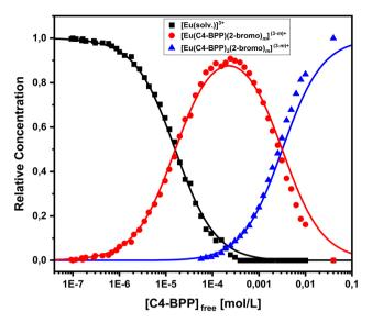
Fig. 9 Relative Eu(III) species concentrations in methanol containing 1.5 vol% water and 5.0  $\times$   $10^{-1}$  mol L $^{-1}$  2-bromohexanoic acid as a function of the free C4-BPP concentration. Symbols denote experimental data, while lines are calculated using  $\log \beta_1^{'}=4.8$  and  $\log \beta_2^{'}=7.3$ .  $T=293\,$  K (2-bromohexanoate is abbreviated as 2-bromo).
