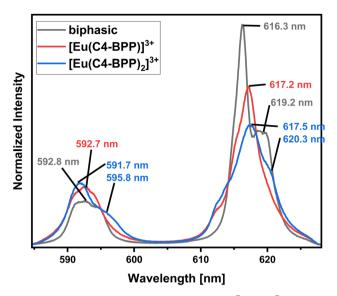
Fig. 7 Normalized fluorescence spectra of the  $^7F_1$  and  $^7F_2$  emission bands of Eu(III) in the organic phase after extraction (black), [Eu(C4 BPP)] $^{3+}$  complex (red) and [Eu(C4 BPP) $_2$ ] $^{3+}$  complex (blue) in methanol containing 1.5 vol% water. Organic phase  $1.0 \times 10^{-2}$  mol L $^{-1}$  C4-BPP and  $5.0 \times 10^{-1}$  mol L $^{-1}$  2-bromohexanoic acid in TPH/1-octanol (10 vol%). Aqueous phase  $3.0 \times 10^{-1}$  mol L $^{-1}$  nitric acid. A/O = 1. T=293 K.
