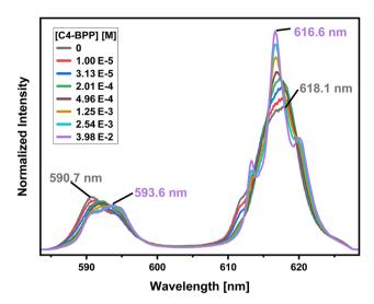
Fig. 8 Normalized fluorescence spectra of the  $^7\text{F}_1$  and  $^7\text{F}_2$  emission bands of Eu(III) in methanol containing 1.5 vol% water and 5.0  $\times$   $10^{-1}$  mol L $^{-1}$  2-bromohexanoic acid as a function of the C4-BPP concentration. [Eu(III)]  $_{\text{ini}}=1.0\times10^{-5}$  mol L $^{-1}$ , [C4-BPP] = (0-3.98)  $\times$   $10^{-2}$  mol L $^{-1}$ . T=293 K.
