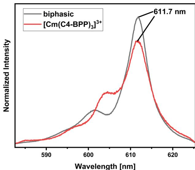
Fig. 6 Normalized fluorescence spectra of Cm(III) in the organic phase after extraction (black) and the  $[\text{Cm}(\text{C4-BPP})_3]^{3+}$  complex (red) in methanol containing 1.5 vol% water. Organic phase  $1.0 \times 10^{-2} \text{ mol L}^{-1}$  C4-BPP and  $5.0 \times 10^{-1} \text{ mol L}^{-1}$  2-bromohexanoic acid in TPH/1-octanol (10 vol%). Aqueous phase  $3.0 \times 10^{-1} \text{ mol L}^{-1}$  nitric acid. A/O = 1.  $T = 293 \text{ K}$ .
