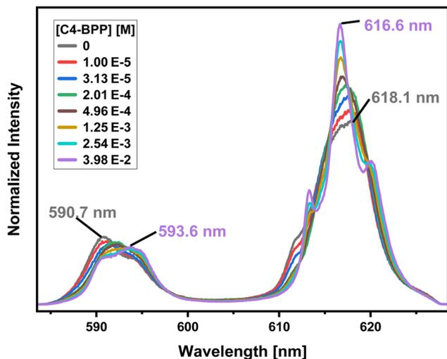
Fig. 8 Normalized fluorescence spectra of the  ${}^7F_1$  and  ${}^7F_2$  emission bands of Eu(III) in methanol containing 1.5 vol% water and  $5.0 \times 10^{-1} \text{ mol L}^{-1}$  2-bromohexanoic acid as a function of the C4-BPP concentration.  $[\text{Eu(III)}]_{\text{ini}} = 1.0 \times 10^{-5} \text{ mol L}^{-1}$ ,  $[\text{C4-BPP}] = (0-3.98) \times 10^{-2} \text{ mol L}^{-1}$ .  $T = 293 \text{ K}$ .
