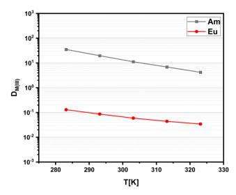
Fig. 5 Distribution ratios for the extraction of Am(III) and Eu(III) with C4-BPP as a function of the temperature organic phase 1.0  $\times$   $10^{-2}$  mol L $^{-1}$  C4-BPP and  $5.0\times10^{-1}$  mol L $^{-1}$ 2-bromohexanoic acid in TPH/1-octanol (10 vol%). Aqueous phase 1.0  $\times$  10 $^{-1}$  mol L $^{-1}$  nitric acid. A/O = 1. T=283-323 K.
