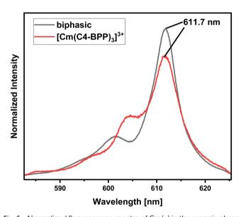
Fig. 6 Normalized fluorescence spectra of Cm(III) in the organic phase after extraction (black) and the [Cm(C4 BPP)3]  $^{3+}$  complex (red) in methanol containing 1.5 vol% water. Organic phase 1.0  $\times$   $10^{-2}$  mol L $^{-1}$  C4-BPP and 5.0  $\times$   $10^{-1}$  mol L $^{-1}$  2-bromohexanoic acid in TPH/1-octanol (10 vol%). Aqueous phase 3.0  $\times$   $10^{-1}$  mol L $^{-1}$  nitric acid. A/O = 1. T=293 K.
