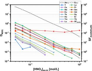
Fig. 2 Distribution ratios for the extraction of Am(III) and Eu(III) ( $\gamma$ , open symbols) and Ln(III) (ICP-MS, solid symbols) with C4-BPP. Organic phase 1.0  $\times$  10<sup>-2</sup> mol L<sup>-1</sup> C4-BPP and 5.0  $\times$  10<sup>-1</sup> mol L<sup>-1</sup> 2-bromohexanoic acid in TPH/1-octanol (10 vol%). Aqueous phase 5.0  $\times$  10<sup>-2</sup> – 1.00 mol L<sup>-1</sup> nitric acid. A/O = 1. T = 293 K.
