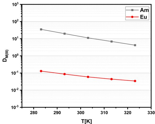
Fig. 5 Distribution ratios for the extraction of Am(III) and Eu(III) with C4-BPP as a function of the temperature organic phase  $1.0 \times 10^{-2} \text{ mol L}^{-1}$  C4-BPP and  $5.0 \times 10^{-1} \text{ mol L}^{-1}$  2-bromohexanoic acid in TPH/1-octanol (10 vol%). Aqueous phase  $1.0 \times 10^{-1} \text{ mol L}^{-1}$  nitric acid. A/O = 1.  $T = 283\text{--}323 \text{ K}$ .
