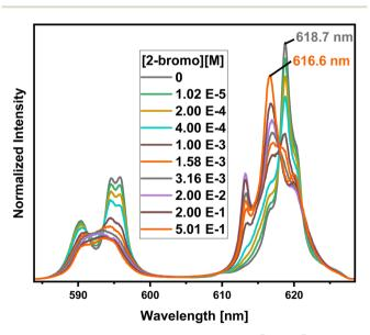
Fig. 10 Normalized fluorescence spectra of the  $^7F_1$  and  $^7F_2$  emission bands of Eu(III) in methanol containing 1.5 vol% water and 3.98  $\times$   $10^{-2}$  mol L $^{-1}$  C4-BPP as a function of the 2-bromohexanoic acid concentration. [Eu(III)] $_{\rm ini}=1.0\times10^{-5}$  mol L $^{-1}$ , [2-bromo] = (0–5.01)  $\times$   $10^{-1}$  mol L $^{-1}$ . T=293 K (2-bromohexanoic acid is abbreviated as 2-bromo).
