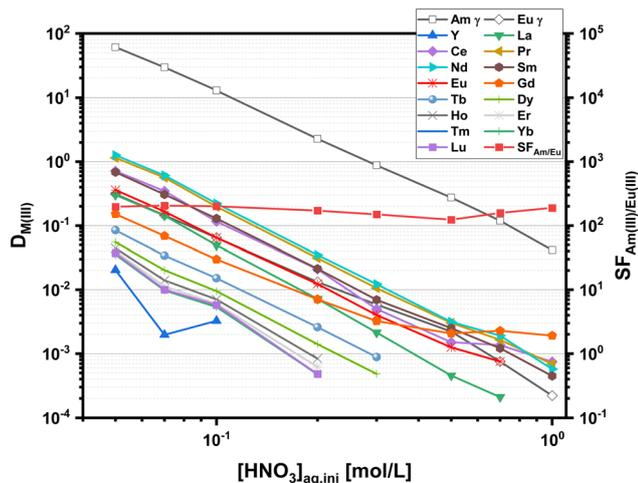
Fig. 2 Distribution ratios for the extraction of Am(III) and Eu(III) ( $\gamma$ , open symbols) and Ln(III) (ICP-MS, solid symbols) with C4-BPP. Organic phase  $1.0 \times 10^{-2}$  mol L $^{-1}$  C4-BPP and  $5.0 \times 10^{-1}$  mol L $^{-1}$  2-bromohexanoic acid in TPH/1-octanol (10 vol%). Aqueous phase  $5.0 \times 10^{-2}$ – $1.00$  mol L $^{-1}$  nitric acid. A/O = 1.  $T = 293$  K.
