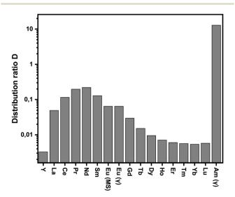
Fig. 3 Distribution ratios for the extraction of Am(III) and Ln(III) with C4-BPP. Organic phase  $1.0\times10^{-2}$  mol L $^{-1}$  C4-BPP and  $5.0\times10^{-1}$  mol L $^{-1}$  2-bromohexanoic acid in TPH/1-octanol (10 vol%). Aqueous phase  $1.0\times10^{-1}$  mol L $^{-1}$  nitric acid. A/O = 1. T=293 K.
