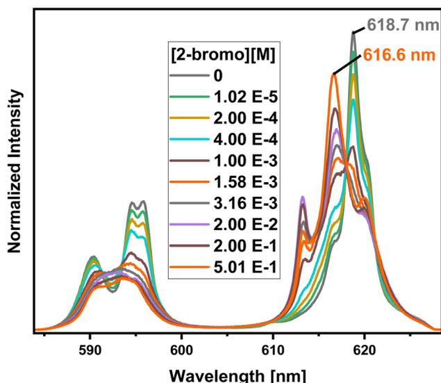
Fig. 10 Normalized fluorescence spectra of the  ${}^7\text{F}_1$  and  ${}^7\text{F}_2$  emission bands of Eu(III) in methanol containing 1.5 vol% water and  $3.98 \times 10^{-2} \text{ mol L}^{-1}$  C4-BPP as a function of the 2-bromohexanoic acid concentration.  $[\text{Eu}(\text{III})]_{\text{ini}} = 1.0 \times 10^{-5} \text{ mol L}^{-1}$ ,  $[\text{2-bromo}] = (0-5.01) \times 10^{-1} \text{ mol L}^{-1}$ .  $T = 293 \text{ K}$  (2-bromohexanoic acid is abbreviated as 2-bromo).
