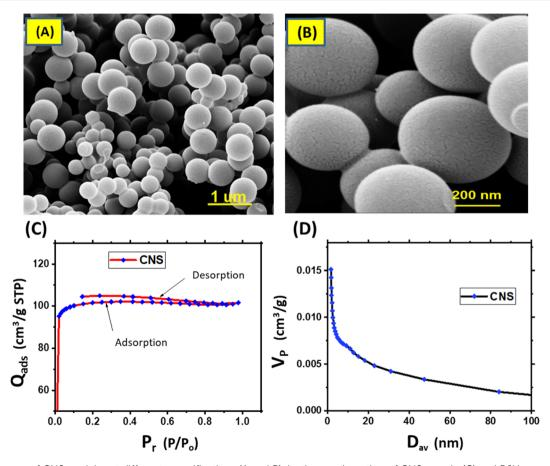
Fig. 2 SEM images of CNS particles at different magnifications (A and B), isotherm adsorption of CNS sample (C) and BJH pore distribution of CNS (D).
