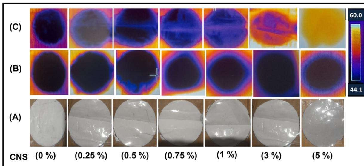
Fig. 5 Photos of the membranes at different concentrations of CNS, (A) photos from an ordinary camera, (B) IR-thermal camera images of the membranes after 1 min. of exposure to sunlight, and (C) IR-thermal camera images of the membranes after 25 min. of exposure to sunlight (note: IR thermal camera photos have been taken outdoor at under direct solar radiation at 1 pm, August, Egypt).
