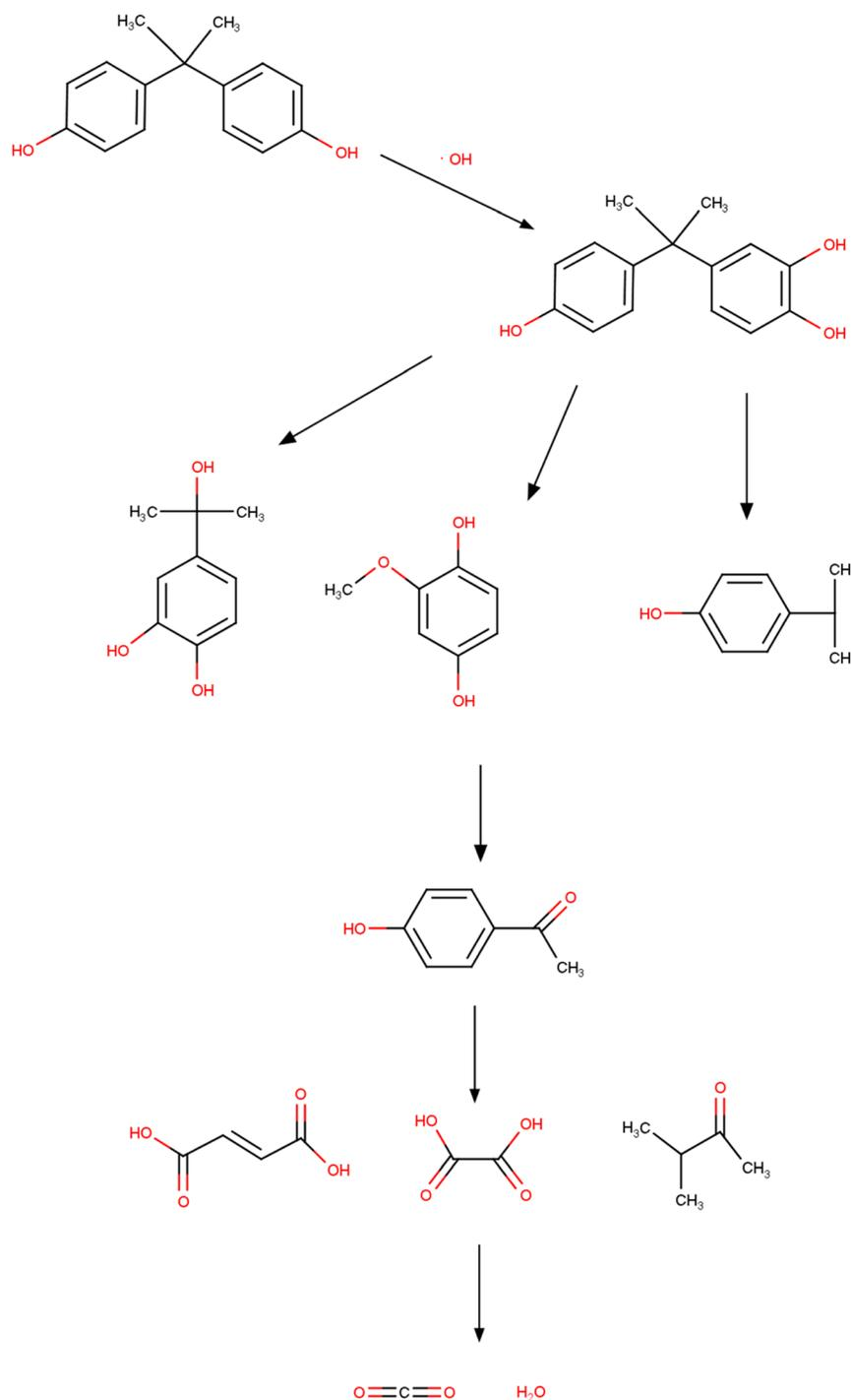
Fig. 7 BPA degradation mechanism for the photo-Fenton reaction.
