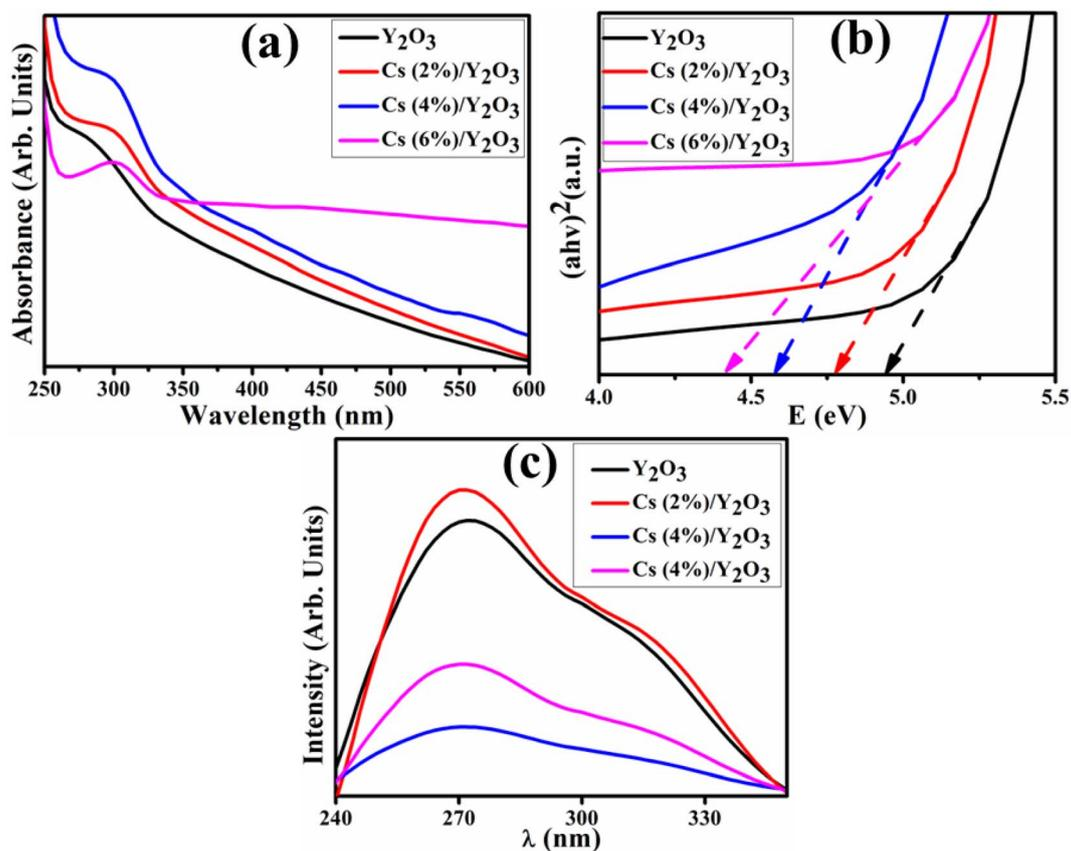
Fig. 4 (a) Absorption spectra, (b) band gap energy, and (c) emission spectra of  $\text{Y}_2\text{O}_3$  and Cs (2, 4, and 6 wt%) doped  $\text{Y}_2\text{O}_3$  NSs.
