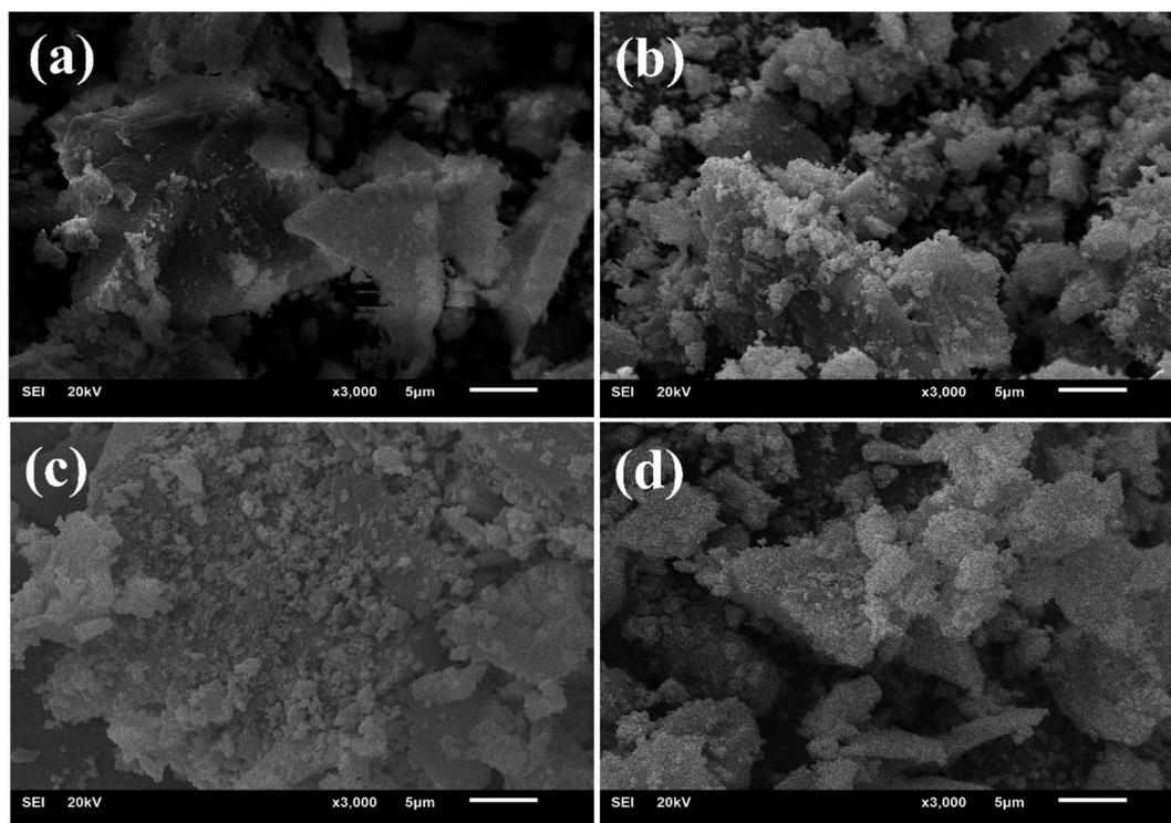
Fig. 5 (a–d) FESEM micrograph of pure and Cs (2, 4 and 6 wt%) doped Y<sub>2</sub>O<sub>3</sub> NSs.
