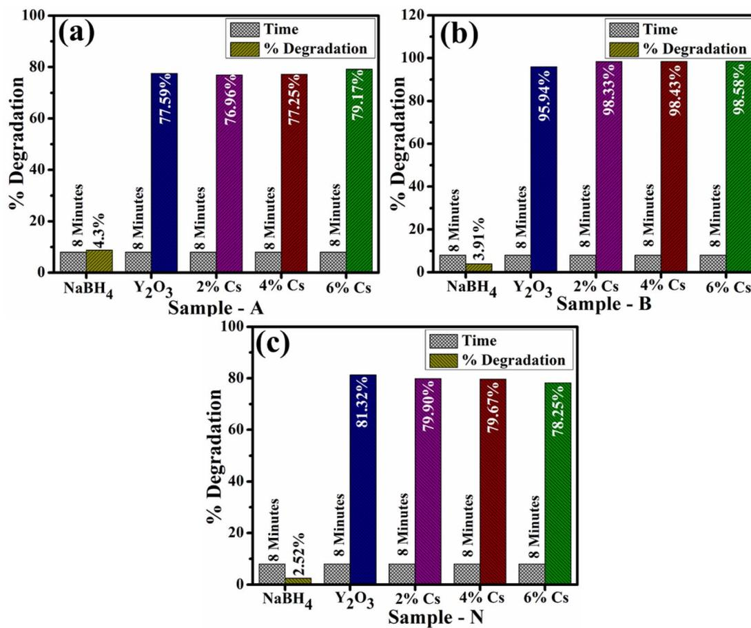
Fig. 8 Catalytic activity of  $\text{Y}_2\text{O}_3$  and Cs- $\text{Y}_2\text{O}_3$  (2, 4, and 6 wt%) in (a) acidic, (b) basic and (c) neutral media.
