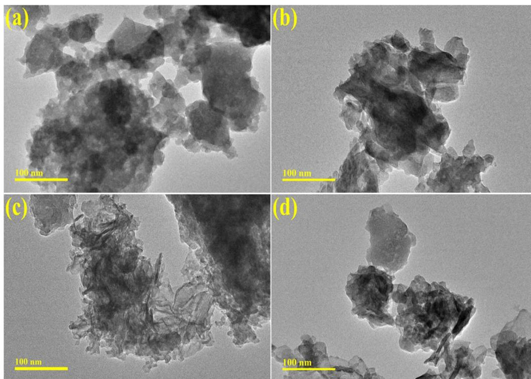
Fig. 6 TEM images (a) Y<sub>2</sub>O<sub>3</sub> and (b–d) Cs (2, 4, and wt%)-doped Y<sub>2</sub>O<sub>3</sub> NSs.
