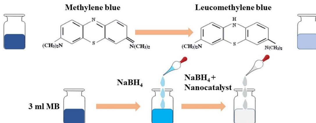
Fig. 2 Mechanism and experimental performance of catalytic activity.
