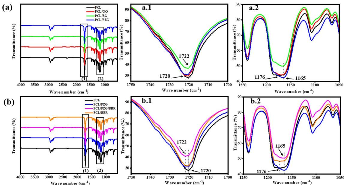
Fig. 2 FTIR spectra of PCL fiber membrane and the composite fiber membranes in the wavenumber ranges from 500 to 4000 (a and b) 1700 to 1750 cm<sup>-1</sup> (a.1 and b.1), and 1050 to 1250 cm<sup>-1</sup> (a.2 and b.2).
