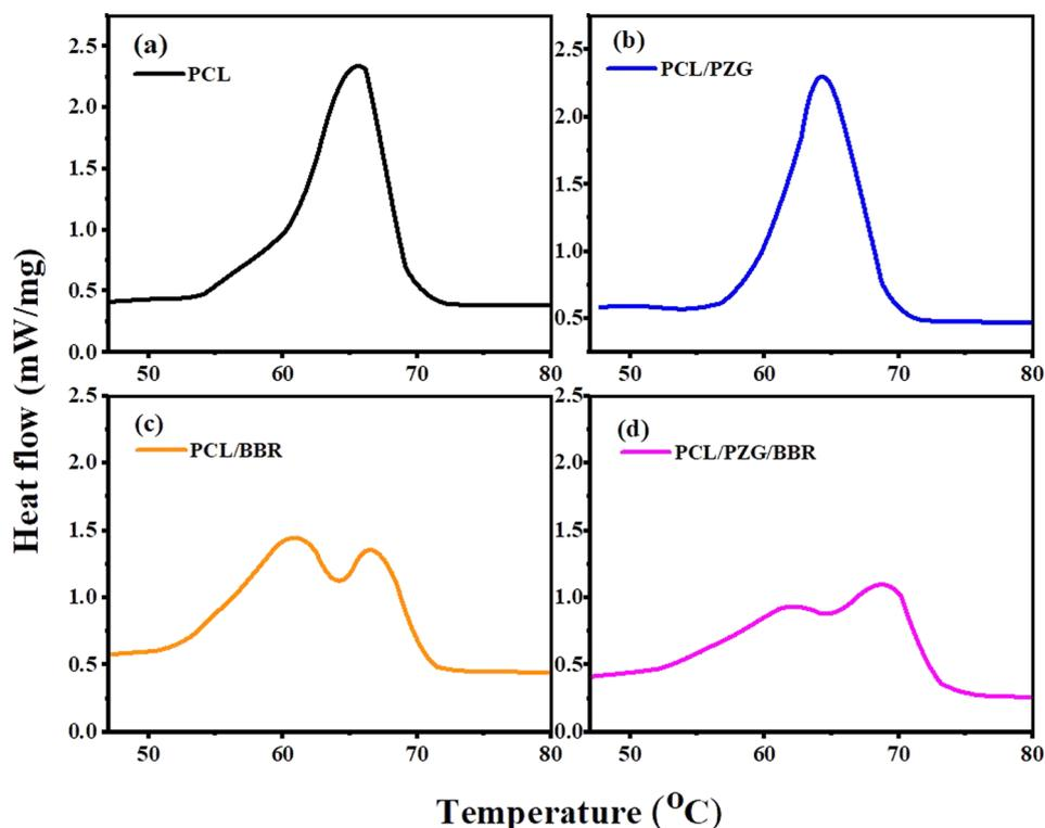
Fig. 4 DSC curves of (a) PCL, (b) PCL/PZG, (c) PCL/BBR, and (d) PCL/PZG/BBR membranes.
