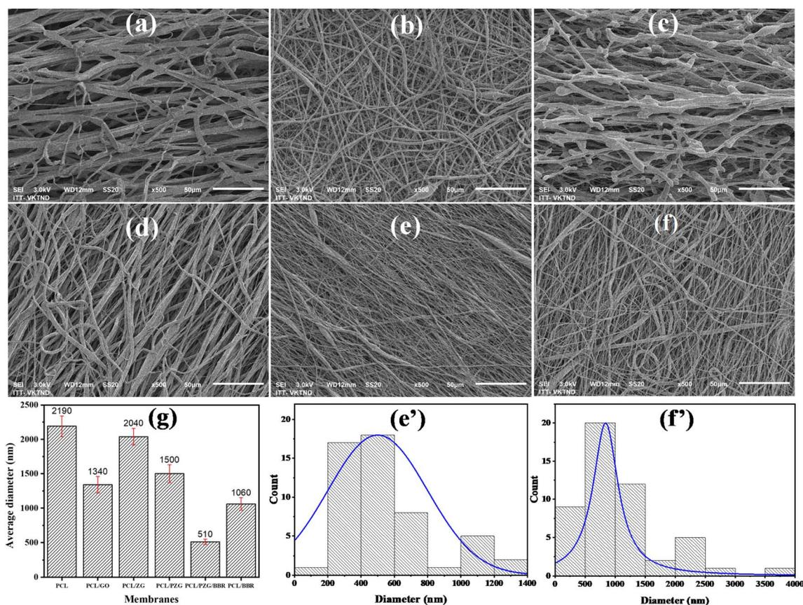
Fig. 1 SEM images of electrospun (a) PCL, (b) PCL/GO, (c) PCL/ZG, (d) PCL/PZG, (e) PCL/PZG/BBR, and (f) PCL/BBR fibers, average diameter of the fibers (g), and diameter distributions of electrospun (e') PCL/PZG/BBR and (f') PCL/BBR fibers.
