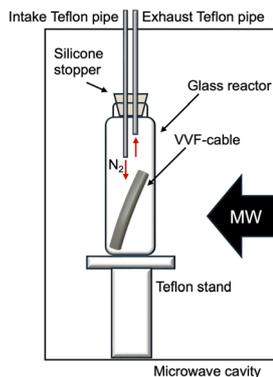
Fig. 2 Illustrative image of a microwave cavity with a reactor containing a VVF cable.
