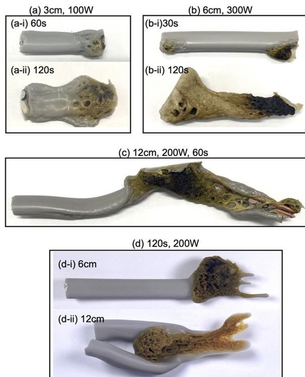
**Fig. 7** Photographs of the pyrolysis of VVF cable by microwave irradiation under various conditions. (a) 3 cm VVF cable length irradiated with 200 and 300 W microwaves, (b) 9 cm VVF cable length irradiated with 200 and 300 W microwaves, (c and d) 18 cm VVF cable length irradiated with 100 and 200 W microwaves.
