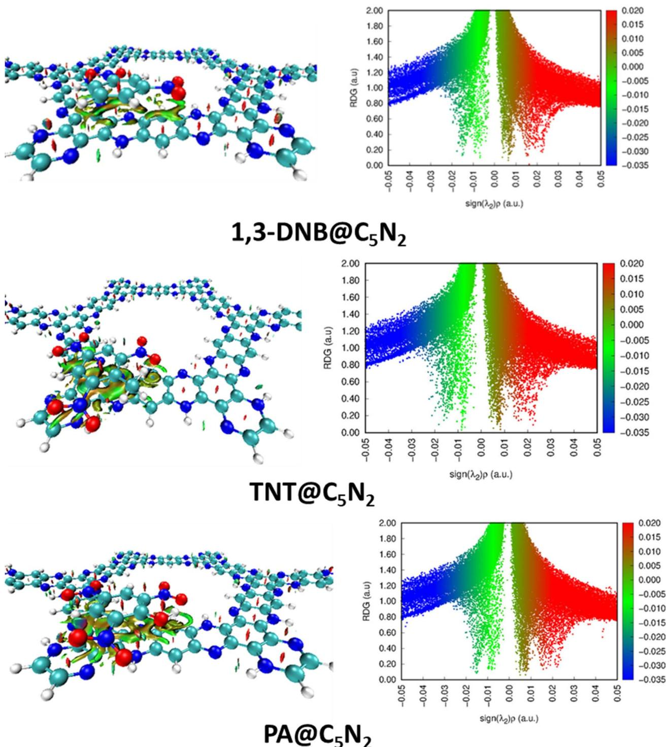
Fig. 4 3D isosurface and 2D RDG graph of nitroaromatics analytes@C<sub>5</sub>N<sub>2</sub> complexes.
