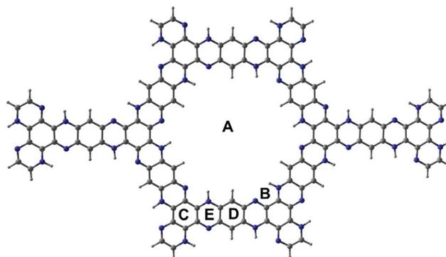
Fig. 1 Optimised geometry of  $C_5N_2$  at PBE0-D3BJ/def2SVP with five binding sites *i.e.*, central cavity (A), triazine site (B), benzene ring (C), hydrogenated benzene ring (D) and pyrazine ring (E). Blue color shows the nitrogen atom, grey shows the carbon atom and greyish-white shows the hydrogen atom.
