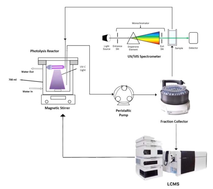
Fig. 1 Experimental setup for MEA breakdown via UV/H<sub>2</sub>O<sub>2</sub> photolysis.
