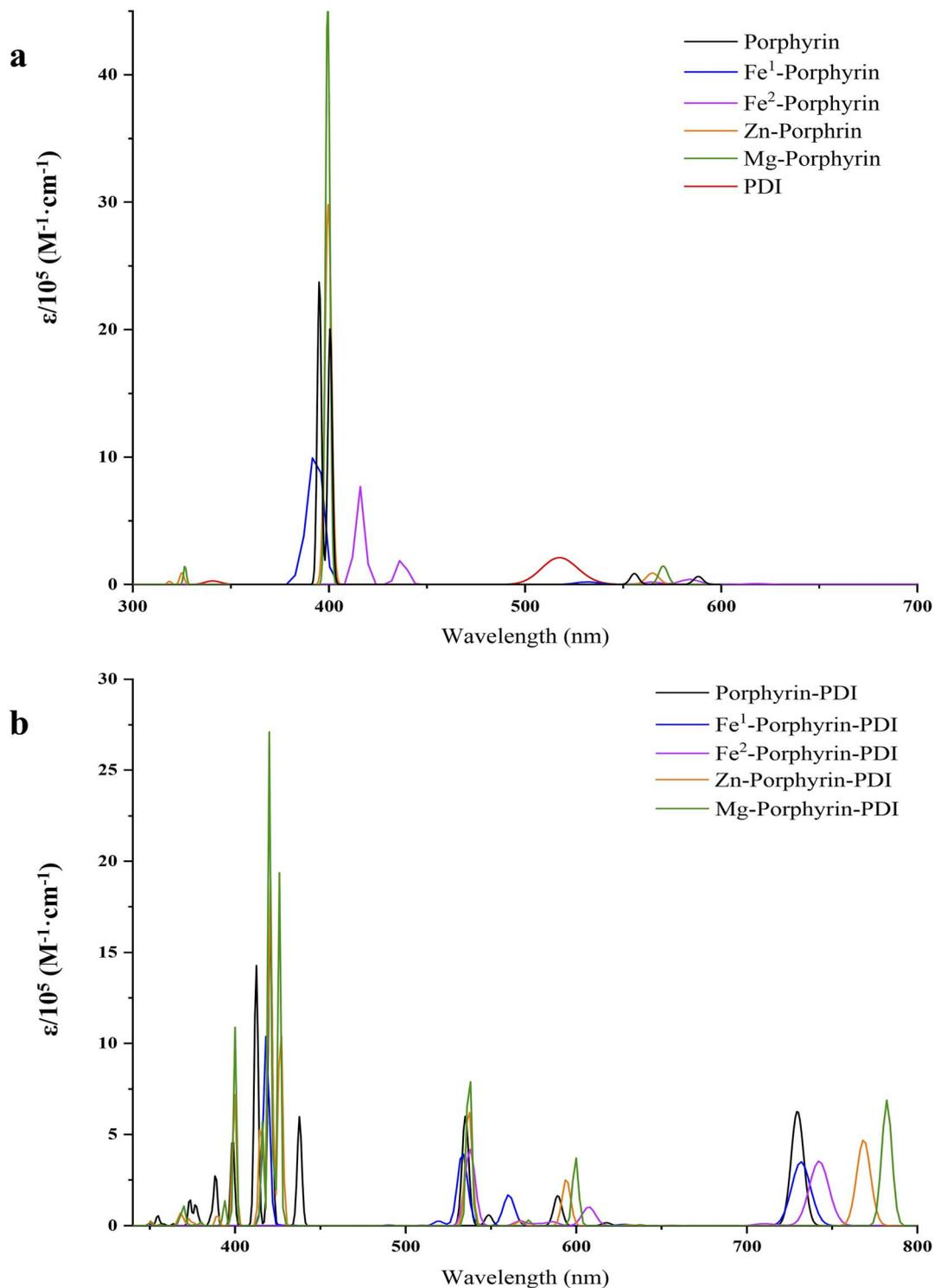
Fig. 4 Simulated absorption spectra of (a) M-porphyrin and (b) M-porphyrin-PDI.
