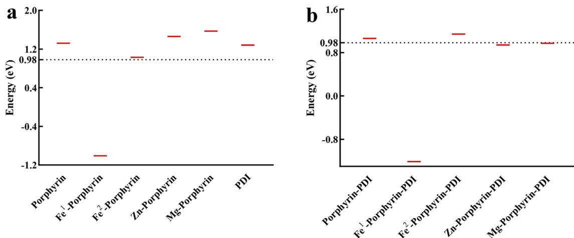
Fig. 6 Triplet excitation energies for (a) M-porphyrin and (b) M-porphyrin-PDI. The energy line of 0.98 eV, required to activate molecular oxygen, was highlighted as the black dashed line.
