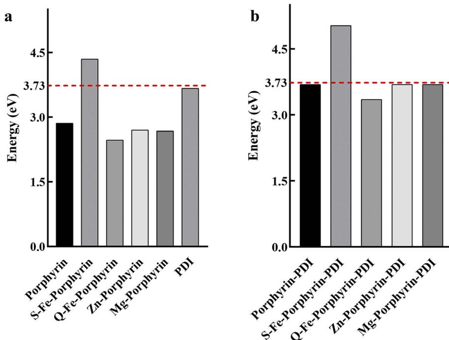
Fig. 5 Adiabatic electron affinities for (a) M-porphyrin and (b) M-porphyrin-PDI. The energy line of 3.73 eV for molecular oxygen was highlighted as the red dashed line.
