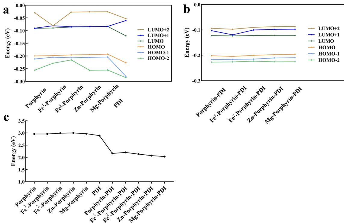
Fig. 3 Calculated frontier molecular orbital energies of ground states of (a) M-porphyrin and (b) M-porphyrin-PDI. (c) LUMO–HOMO energy gap.
