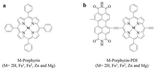
Scheme 1 Molecular structures of (a) M-porphyrin and (b) M-porphyrin-PDI. Fe<sup>1</sup>: singlet state; Fe<sup>2</sup>: quintet state.
