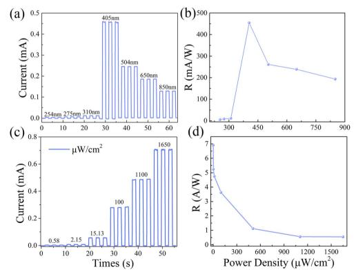
Fig. 5 (a) *I*-*t* curves of the CPB@BPB/T-Si detector under the same power and different wavelength laser irradiation. (b) Responsiveness curve of the device under different wavelength illumination; (c) *I*-*t* curves of the CPB@BPB/T-Si detector under different power of 405 nm wavelength laser illumination; (d) responsiveness curve of the device under different power of illumination.
