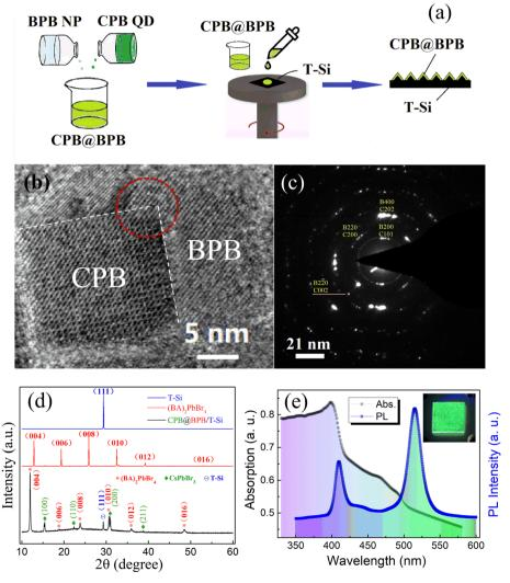
Fig. 2 (a) Schematic illustration of the fabrication of CPB@BPB HSs and CPB@BPB film on T-Si substrate. (b) HRTEM, and (c) SAED pattern of the CPB@BPB HSs. (d) XRD patterns of the pristine (BA)<sub>2</sub>PbBr<sub>4</sub> powder, the silicon substrate and the CPB@BPB film. (e) Optoelectronic properties of CPB@BPB HS.
