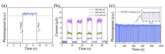
Fig. 6 (a) Response time of the CPB@BPB/T-Si photodetector; (b) *I-t* curves of photocurrent under different light intensities; (c) recyclable switching operation of photocurrent response.
