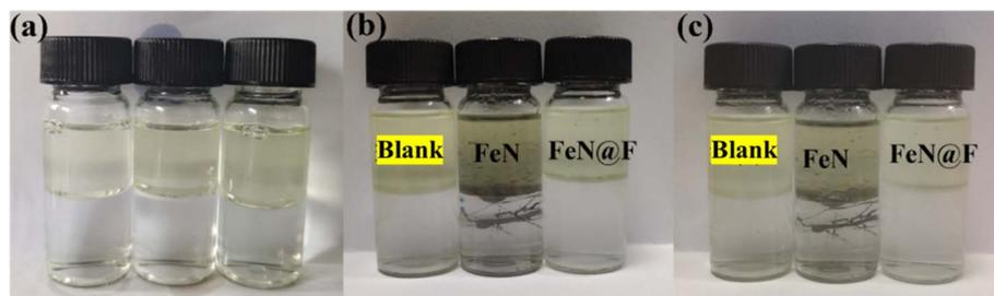
Fig. 6 Interfacial activity of blank group,  $\text{Fe}_3\text{N}$ , and  $\text{Fe}_3\text{N@F}$  (a) before shaking; (b) after shaking and standing for 20 min; (c) after shaking and standing for 24 h.
