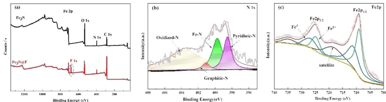
Fig. 3 X-ray photoelectron spectroscopy (XPS) spectra of (a) full spectrum of composite materials; (b)  $\text{Fe}_3\text{N}$  and (c)  $\text{Fe}_3\text{N}@F$ .
