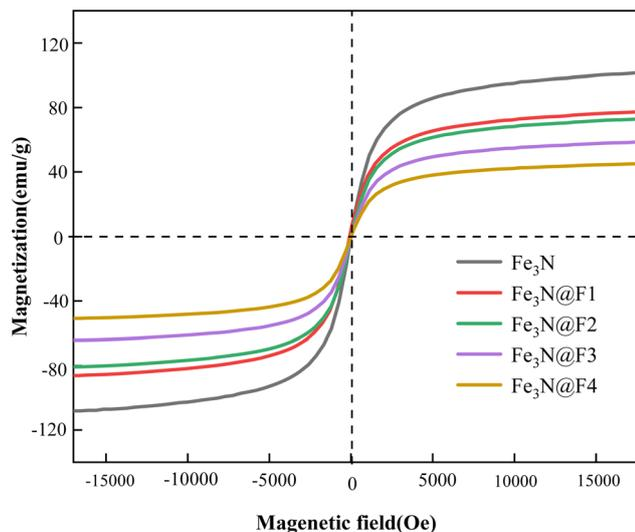
Fig. 9 Magnetization hysteresis loops of  $\text{Fe}_3\text{N}$  and  $\text{Fe}_3\text{N@F}$  demulsifier.
