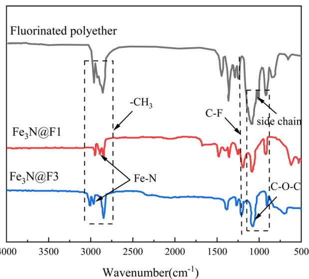
Fig. 4 FTIR spectra of fluoroether and  $\text{Fe}_3\text{N}@F$ .
