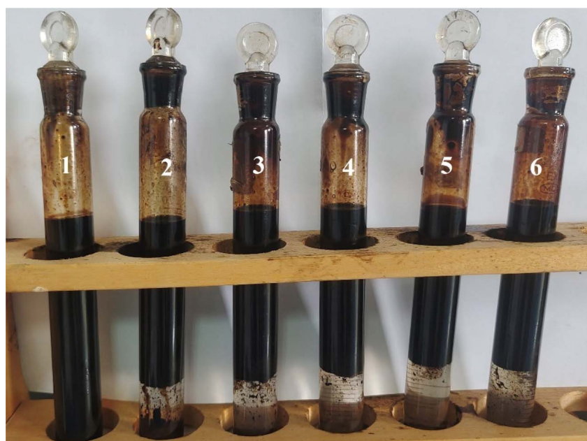
Fig. 10 The demulsification effects of different materials on crude oil emulsions.
