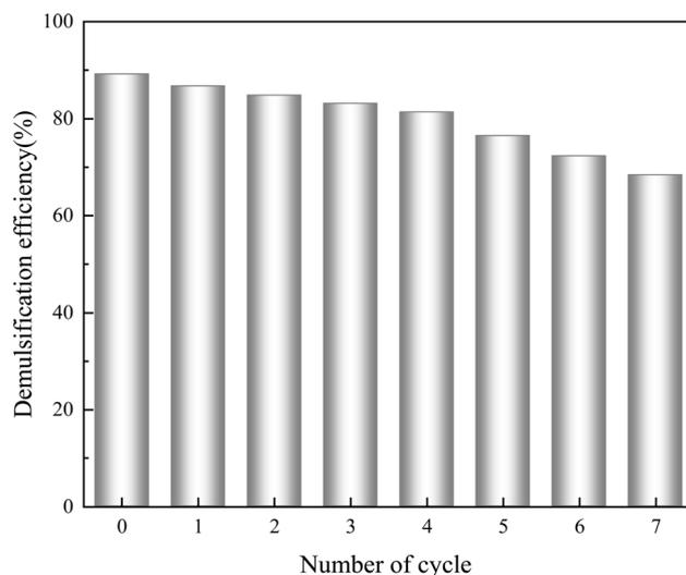
Fig. 14 The demulsification efficiency of  $\text{Fe}_3\text{N@F}$  at various cycling intervals.
