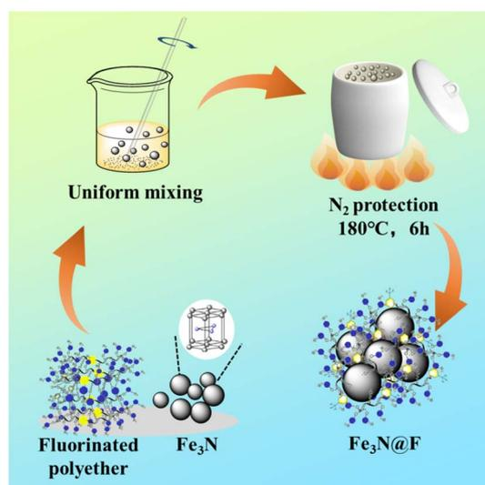
Fig. 1 Synthesis route of Fe<sub>3</sub>N@F.
