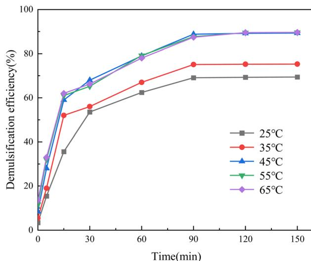
Fig. 13 Effects of the varying demulsification temperatures and sedimentation durations of  $\text{Fe}_3\text{N@F}_3$  for the demulsification of crude oil emulsions.
