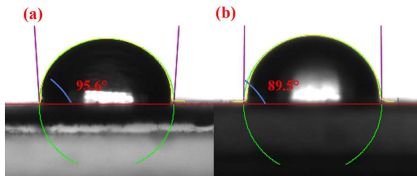
Fig. 8 Three-phase contact angles of (a) Fe<sub>3</sub>N and (b) Fe<sub>3</sub>N@F.
