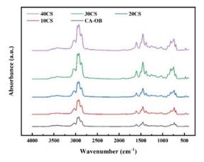
Fig. 5 FTIR spectra of the pyrolysis oil for CA-OB/CS blends.
