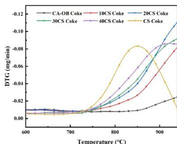
Fig. 10 The rate curves of CO<sub>2</sub> gasification for the cokes of CA-OB/CS blends.Table 8 Initial temperatures of CO<sub>2</sub> gasification for the cokes of CA-OB/CS blends
