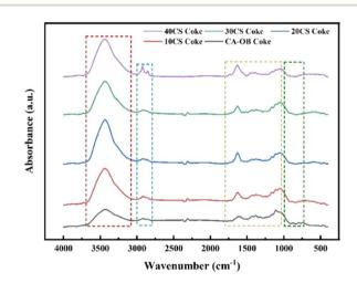
**Fig. 8** FTIR spectra of the cokes from the co-pyrolysis of CA-OB and CS.
