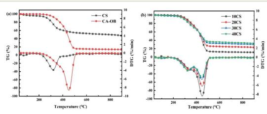
Fig. 1 TG and DTG curves of CS, CA-OB, and their blends under different ratios.
