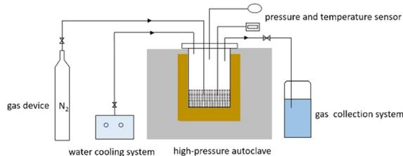
Scheme 1 Schematic diagram of the co-pyrolysis system.
