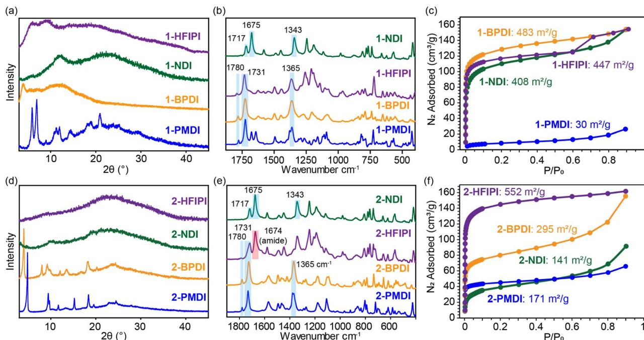
**Fig. 1** (a) Overlay of PXRD patterns of 1-XDI MOFs. (b) Overlay of ATR-IR spectra of 1-XDI MOFs. Characteristic imide IR bands are highlighted in blue. (c)  $N_2$  adsorption isotherms for 1-XDI MOFs measured at 77 K. (d) Overlay of PXRD patterns of 2-XDI MOFs. (e) Overlay of ATR-IR spectra of 2-XDI MOFs. Characteristic imide IR bands are highlighted in blue. (f)  $N_2$  adsorption isotherms for 2-XDI MOFs measured at 77 K.
