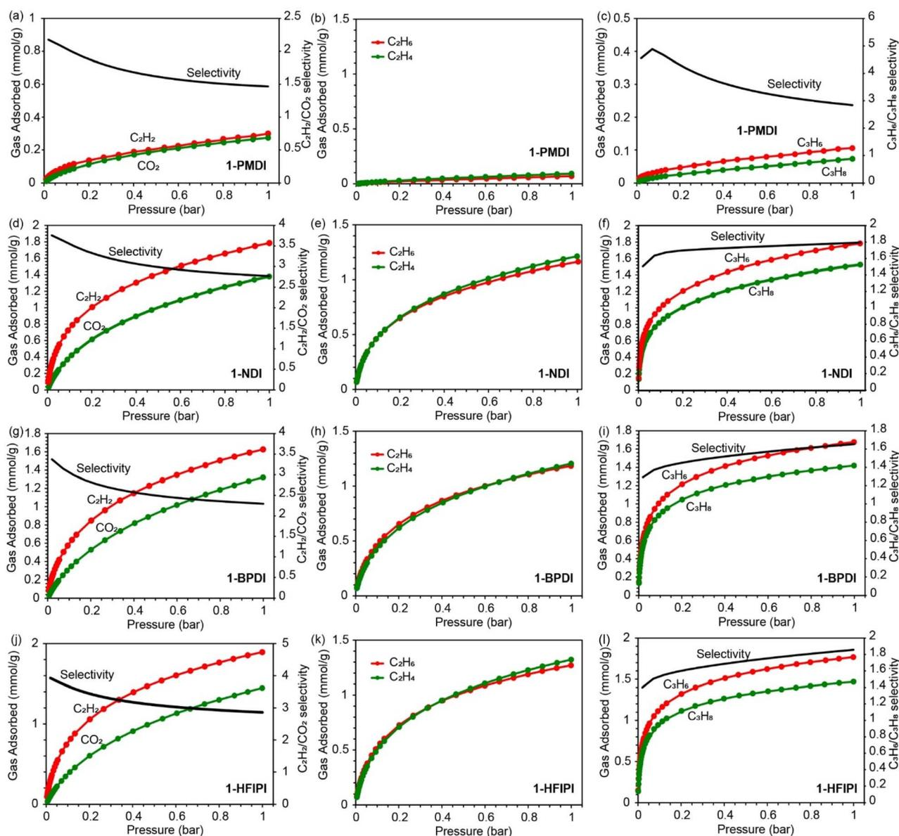
Fig. 3 (a)–(l) C<sub>2</sub>H<sub>2</sub> and CO<sub>2</sub>, C<sub>2</sub>H<sub>4</sub> and C<sub>2</sub>H<sub>6</sub>, C<sub>3</sub>H<sub>6</sub> and C<sub>3</sub>H<sub>8</sub> adsorption isotherms (left y-axis) and predicted IAST selectivity at 300 K (right y-axis) for **1-XDI** MOFs.
