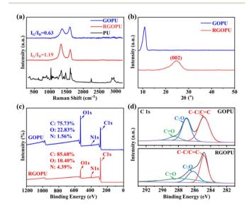
Fig. 2 Chemical structure and composition of RGOPU. (a) Raman spectra of the RGOPU, GOPU, and PU. (b) XRD spectra of the GOPU and RGOPU. (c) XPS full-spectrum and (d) C 1s high-resolution spectra of the GOPU and RGOPU.
