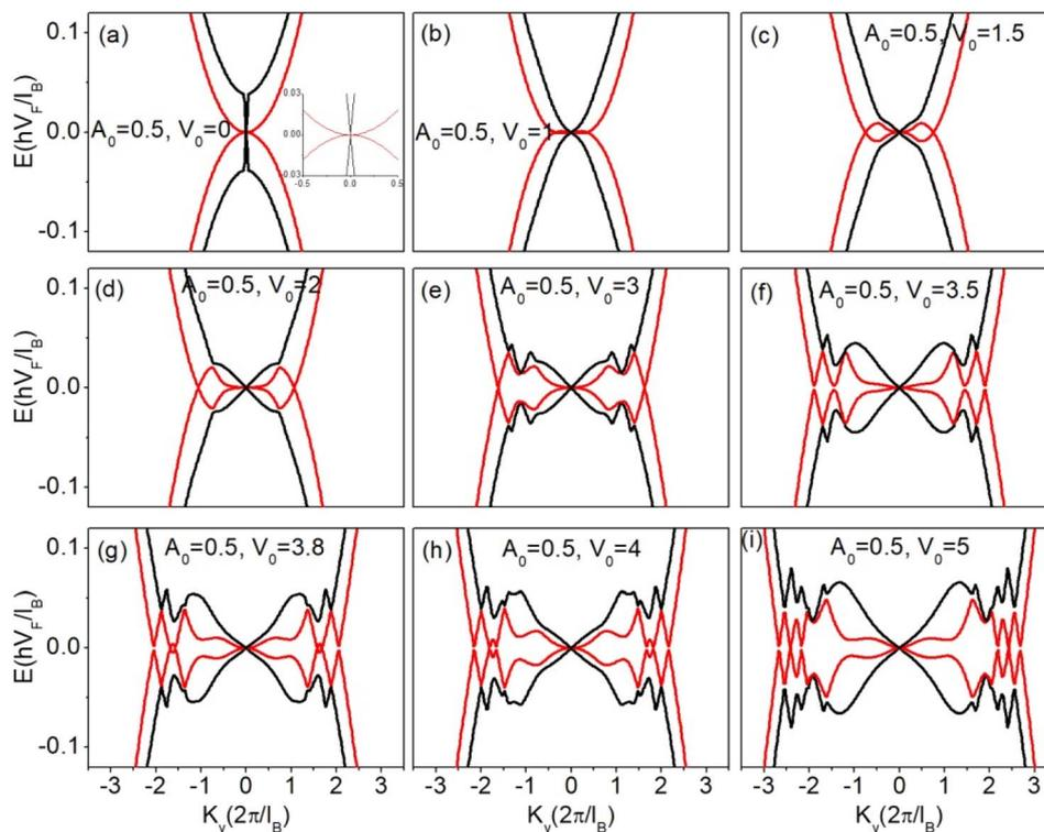
Fig. 8 Energy dispersion along the  $k_y$  direction ( $k_x = 0$ ) with same potential for each layer. The barrier and well widths are equal ( $d_b = d_w = 5$ ,  $L = W = 5$ ,  $d = L + W = d_b + d_w = 10$ ), the barrier height of the vector potential is 0.5 which is constant while the barrier height of the electric potential  $V_0 = 0, 1, 1.5, 2, 3, 3.5, 3.8, 4, 5$  in (a)–(i) respectively.
