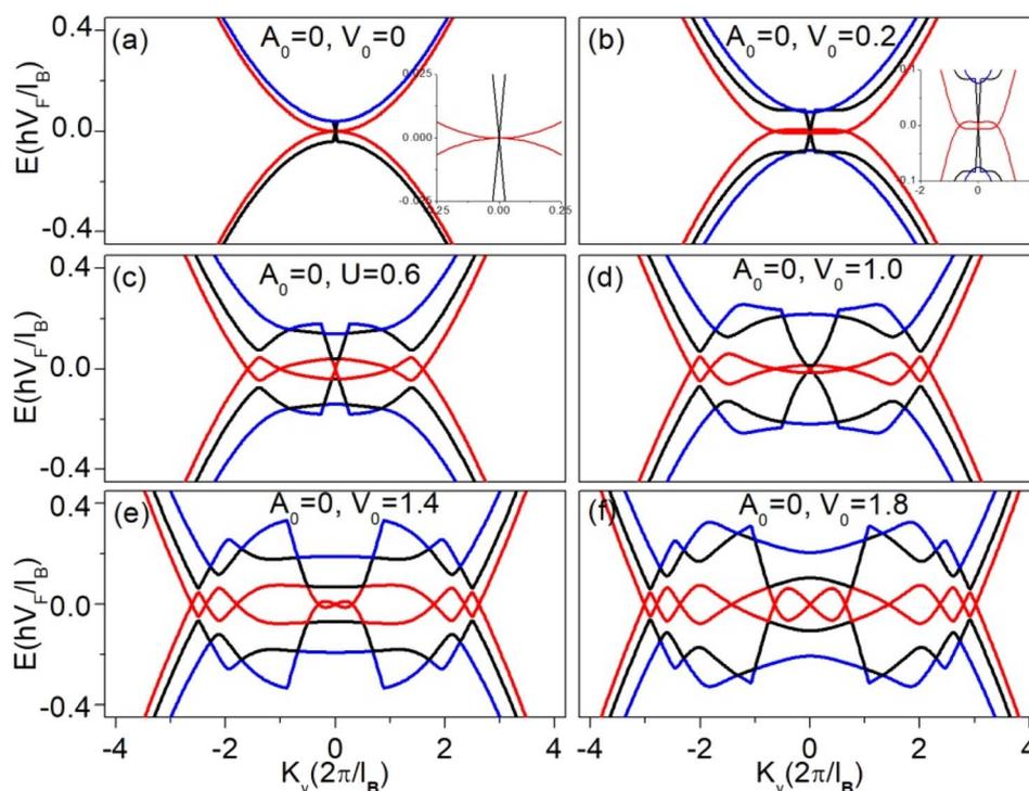
Fig. 5 Energy dispersion along  $k_y$  direction for  $k_x = 0$  for the first three mini-bands, with equal barrier and well widths ( $L = W = 5$ ) and different barrier heights  $V_0 = 0, 0.2, 0.6, 1, 1.4, 1.8$  in (a)–(f) respectively.
