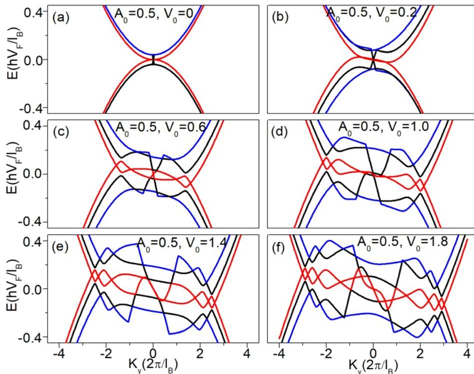
Fig. 6 Energy dispersion along the  $k_y$  direction ( $k_x = 0$ ) with equal barrier and well widths ( $d_b = d_w = 5$ ,  $L = W = 5$ ,  $d = L + W = d_b + d_w = 10$ ). The barrier height of the vector potential is 0.5 which is constant while the barrier height of the electric potential is different. The barrier heights  $V_0 = 0, 0.2, 0.6, 1.0, 1.4, 1.8$  in (a)–(f) respectively.
