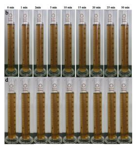
Fig. 6 The real-time images of the flocculation effect of (a) PAFC (b) raw (c) PAFC-10/RS-10 wastewater (d) RS.
