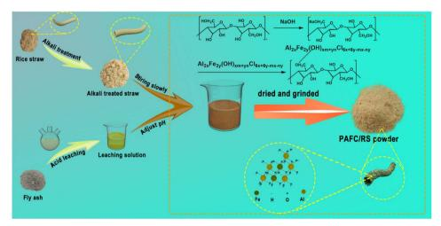
Fig. 1 Schematic for the preparation process of PAFC/RS
