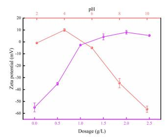
Effect of flocculant dosage and pH on the surface charge of the flocs.
