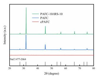
Fig. 4 XRD patterns of PAFC-10/RS-10, PAFC and cPAFC
