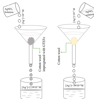
Fig. 10 Removal of [\text{Ag}^+] via cotton wool with and without the impregnation of GTEFe.
