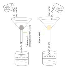
Fig. 10 Removal of [Ag<sup>+</sup>] via cotton wool with and without the impregnation of GTEFe.
