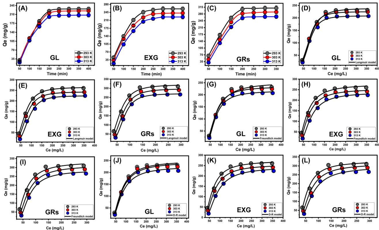
Fig. 6 Experimental impact of starting contents of  $U(vi)$  on its retention performances ((A) (GL), (B) (EXG), and (C) (GRs)), fitting of the retention results with classic Langmuir model ((D) (GL), (E) (EXG), and (F) (GRs)), fitting of the retention results with classic Freundlich model ((G) (GL), (H) (EXG), and (I) (GRs)), and fitting of the retention results with classic D–R model ((J) (GL), (K) (EXG), and (L) (GRs)).
