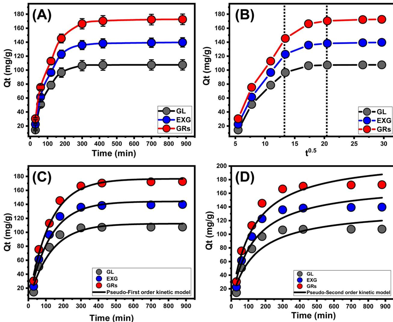
Fig. 5 Experimental impact of contact duration on the retention performances of  $U(vi)$  (A), the plotted intra-particle diffusion curves for the retention of  $U(vi)$  using GL, EXG, and GRs (B), fitting of the determined retention behaviors with pseudo-first order model (C), and fitting of the determined retention behaviors with pseudo-second order model (D).
