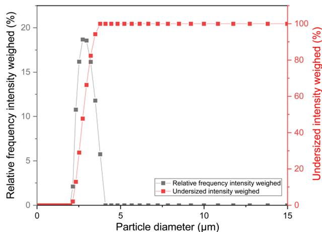
Fig. 3 Particle size determination of anionic resin (PS-DVB-TAC).
