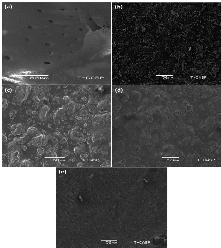
Fig. 4 SEM images of (a) pure PAN membrane (b) [PAN + (PS-DVB-TAC)], (c) [PAN + (PS-DVB-TAC)] + PANI 2 h, (d) [PAN + (PS-DVB-TAC)] + PANI 12 h, and (e) [PAN + (PS-DVB-TAC)] + PANI 24 h.
