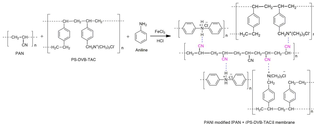
Fig. 1 Proposed route for the synthesis of the composite anion exchange membranes coated with PANI.
