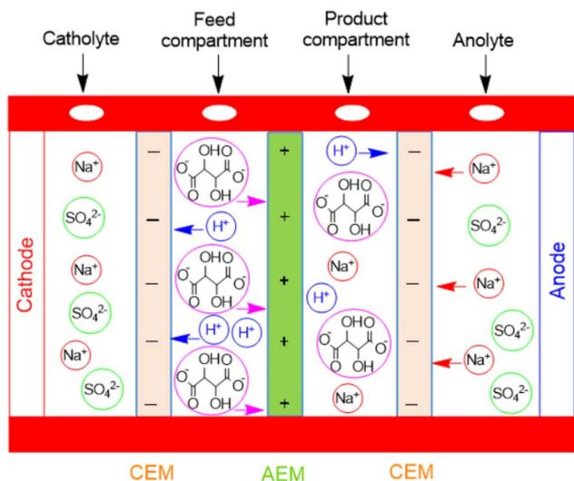
Fig. 2 Experimental setup for the separation of tartaric acid using electro dialysis.
