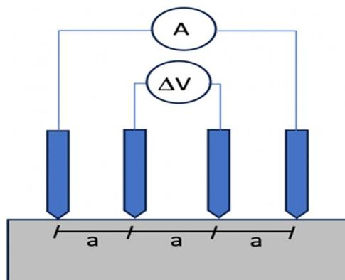
Fig. 10 Concrete resistivity measurement by four electrodes.<sup>83</sup>
