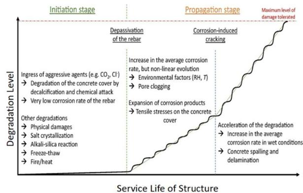
Fig. 1 Schematic representation of the corrosion progression in RC, based on the Tuutti model, with consideration for the service life.<sup>7,9,12</sup>
