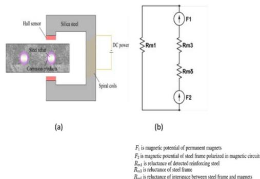
Fig. 5 (a) Electromagnetic corrosion detection device schematic diagram, (b) equivalent model for the electromagnetic set-up.<sup>34,35</sup>
