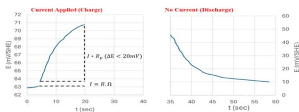
Fig. 12 A graph illustrating the GP measurement of the anodic direction with a  $50 \mu\text{A}$  injection over 30 s, revealing the change in  $\Delta E$  over time throughout the charge and discharge phases.<sup>34</sup>
