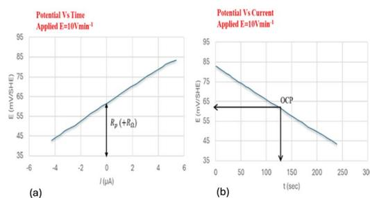
Fig. 13 An illustration of an LPR measurement in relation to OCP in the cathodic direction, from  $\pm 20$  mV. (a) Potential's evolution over time using a potential sweep of  $10 \text{ mV min}^{-1}$ . (b) The potential's evolution with a current during the potential which makes it possible to calculate  $R_p$ .<sup>34</sup>
