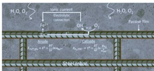
Fig. 2 Corrosion process a schematic view of oxidation and anodic, cathodic reaction.<sup>12</sup>
