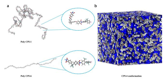
Fig. 3 (a) The molecular chain conformation and repeat unit conformation after structural optimization (C: grey, H: white, O: red, N: blue, F: cyan); (b) fraction free volumes (FFV) of polyimides.
