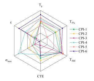
Fig. 10 Comparison of key performance parameters among six polyimides: glass transition temperature,  $T_{\rm g}$ ; the weight loss of 5 wt%,  $T_{\rm 5\%}$ ; optical transmittance at 500 nm,  $T_{\rm 500}$ ; thermal expansion coefficient, CTE; tensile strength,  $\sigma_{\rm max}$ ; dielectric property,  $\varepsilon$ .
